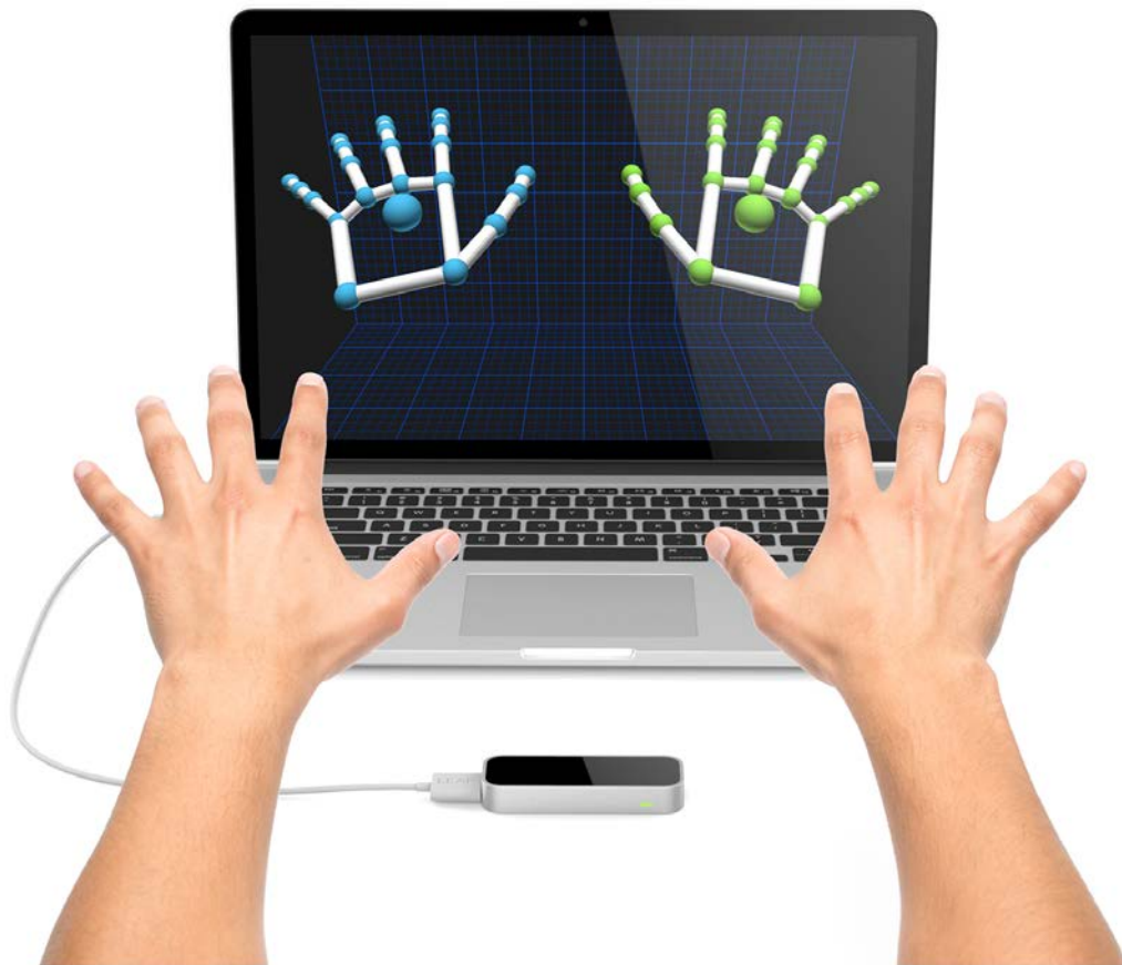
FIGURE 2.9: Leap Motion Hand and Finger Tracker [23].
