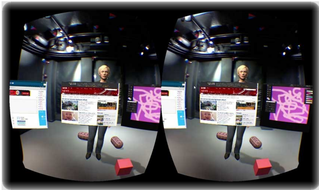
FIGURE 2.4: Stereo Camera Feed with Virtual Objects [11].
