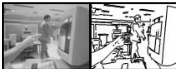
FIGURE 2.6: Edge Detection for Combination with Colour Segmentation [14].
