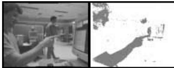
FIGURE 2.5: Colour Segmentation with Background Interference [14].
