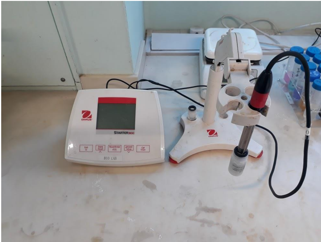
Figure 3. 6 Ohaus Starter 3100 meter for measuring pH
