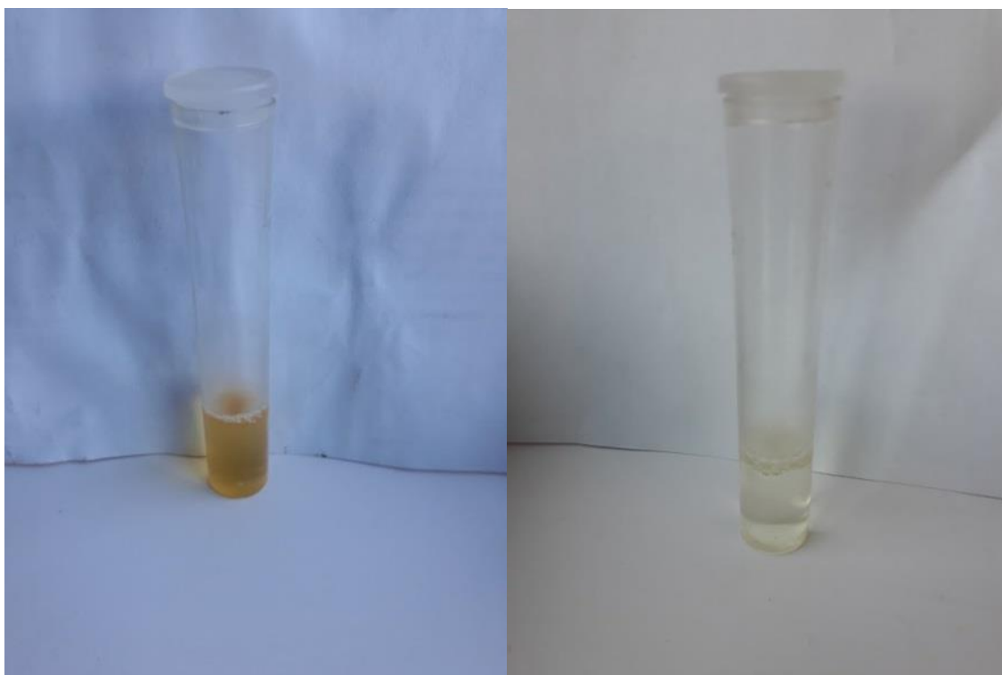
Figure 3. 3 Visual representation of ammonia concentration test in Tetradesmus obliquus grown in unmodified FFW before cultivation (left) and after cultivation (right)
