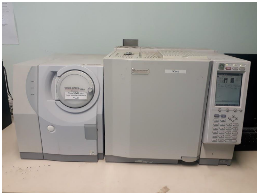
Figure 4. 2 Photo of the GC-MS used for the analysis of biodiesel
