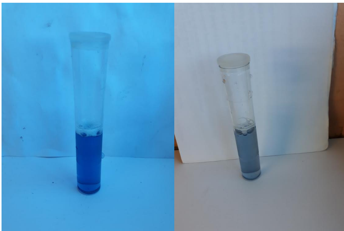
Figure 3. 5 Visual representation of phosphate concentration in Tetradesmus obliquus grown in unmodified FFW before cultivation with higher phosphate concentration (left) and after cultivation with lower phosphate (right)
