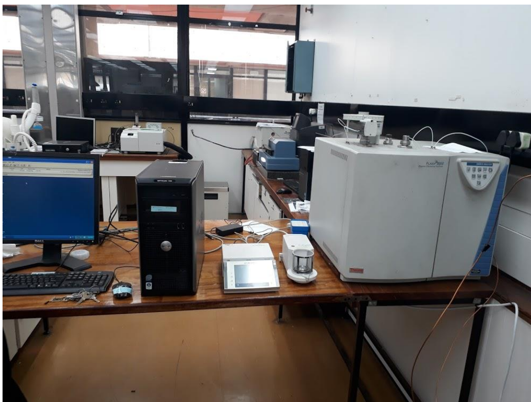
Figure 3. 7 Organic Elemental Analyser for carbon content determination
