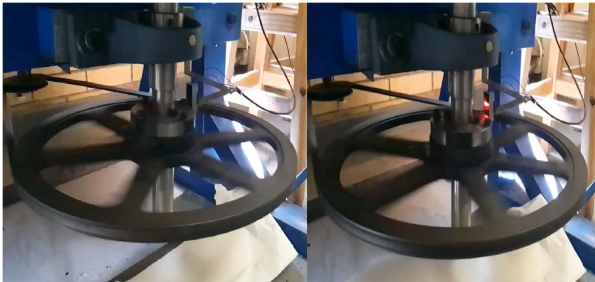
Figure 4. 3: No visual feedback when the IR sensor encounters black surface (on the left) and there is a red visual indication when the sensor encounters the white surface
