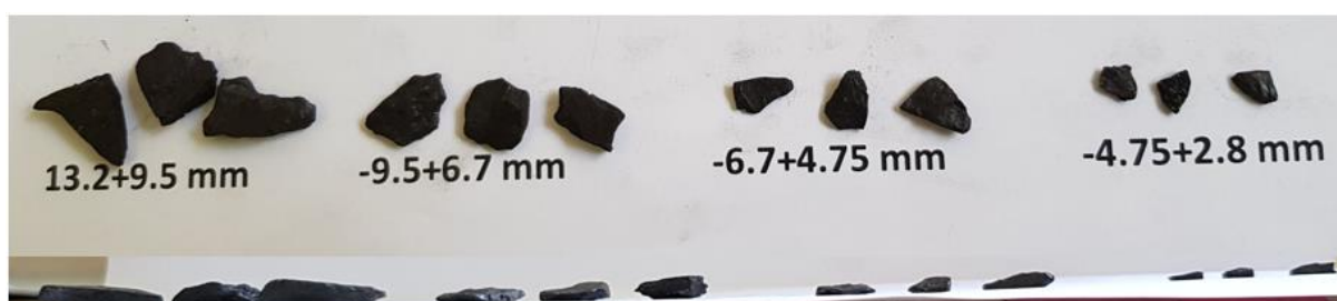
Figure 7. 4: Acicular coal particles from the crusher
