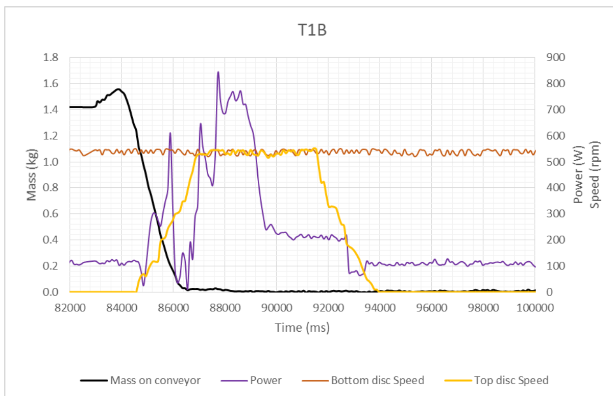
Figure U 2: The signals operating variables for T1B (a repeat of T1A) at the speed of 550 rpm
