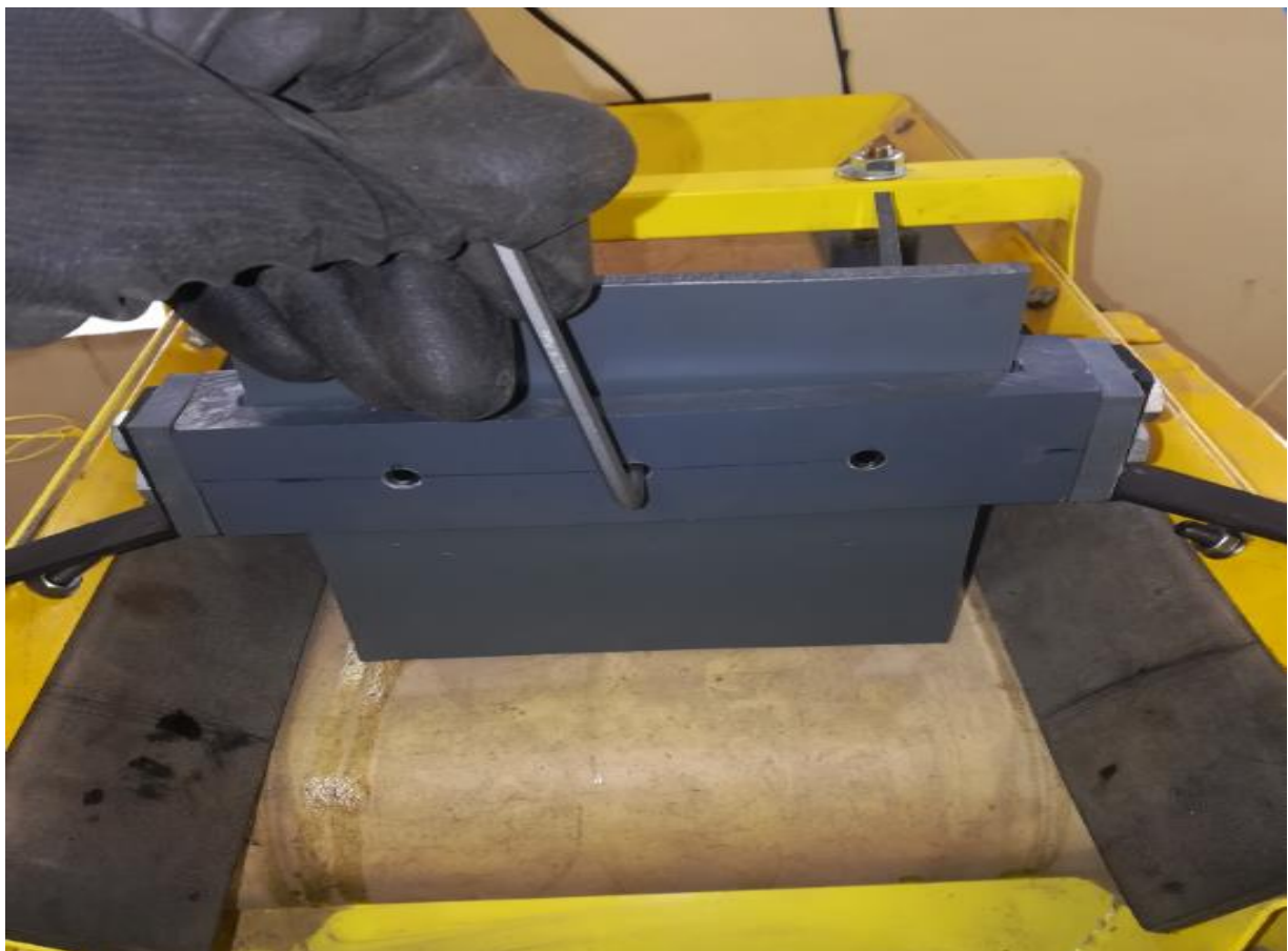
Figure D 2: The grate on the conveyor belt to control the feed rate
