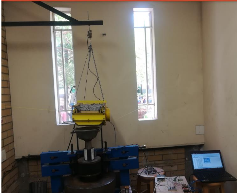
Figure M 1: A conveyor belt with limestone sample (evenly spread) during calibration
