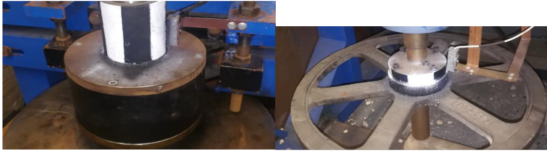
Figure 4. 4: (On the left) The IR sensor placed 1 cm from the shaft of the top disc (with alternating patches of black and white) and (on the right) the IR sensor placed 1 cm from the shaft of the bottom disc (painted in a similar manner)
