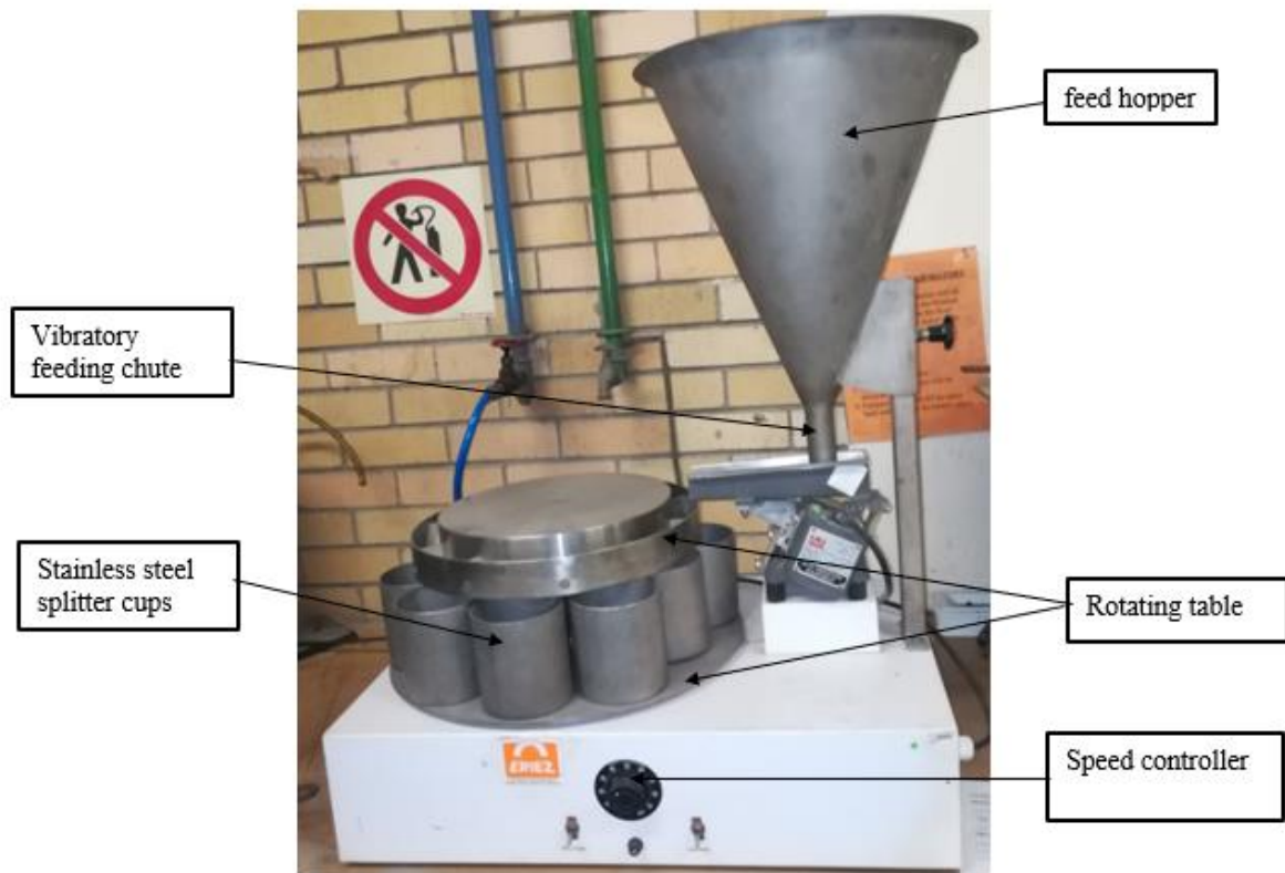
Figure 3. 4: Rotary sampler used to split the samples
