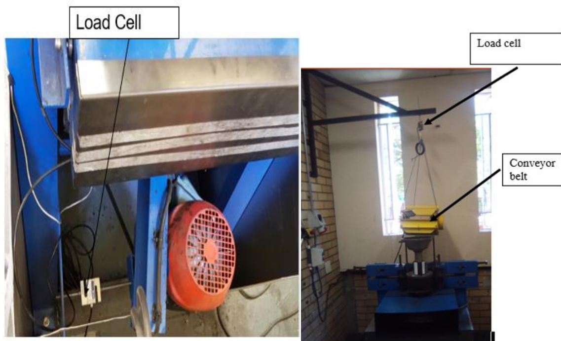
Figure 4. 9: Illustrations of the load cells installed on the crusher to measure the load of the drive system (on the left) and the weight of the materials conveyed to the crusher (on the right)
