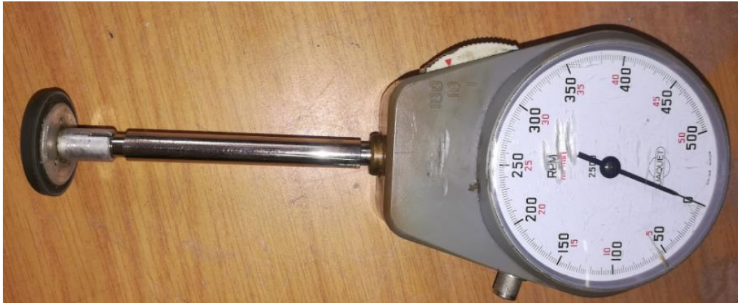
Figure 4. 7: Mechanical hand tachometer type 2200
