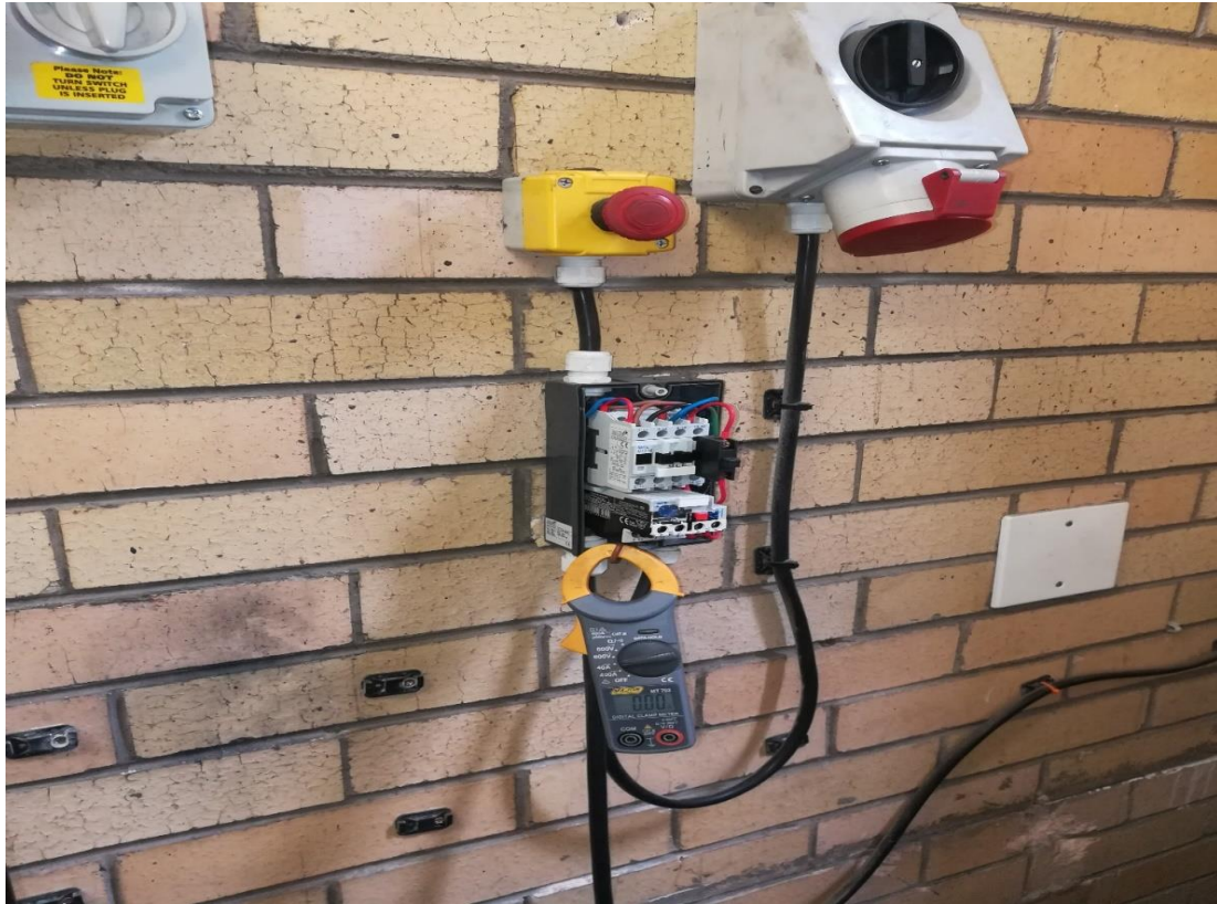
Figure 4. 16: Current measurements for the live wire of the ROC motor using the clamp multi-meter
