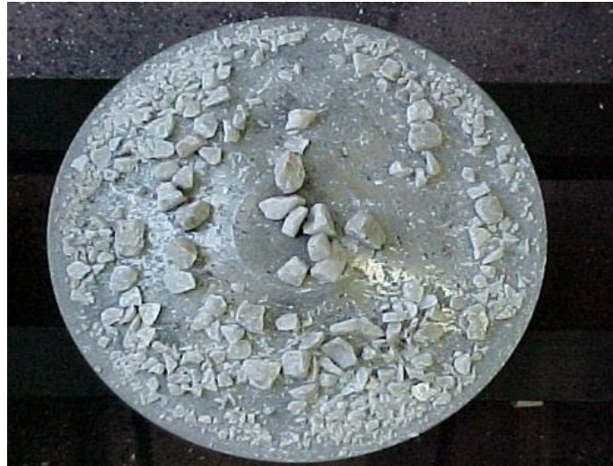
Figure 1. 2: Particle size distribution on the lower disc of the rotary offset crusher
