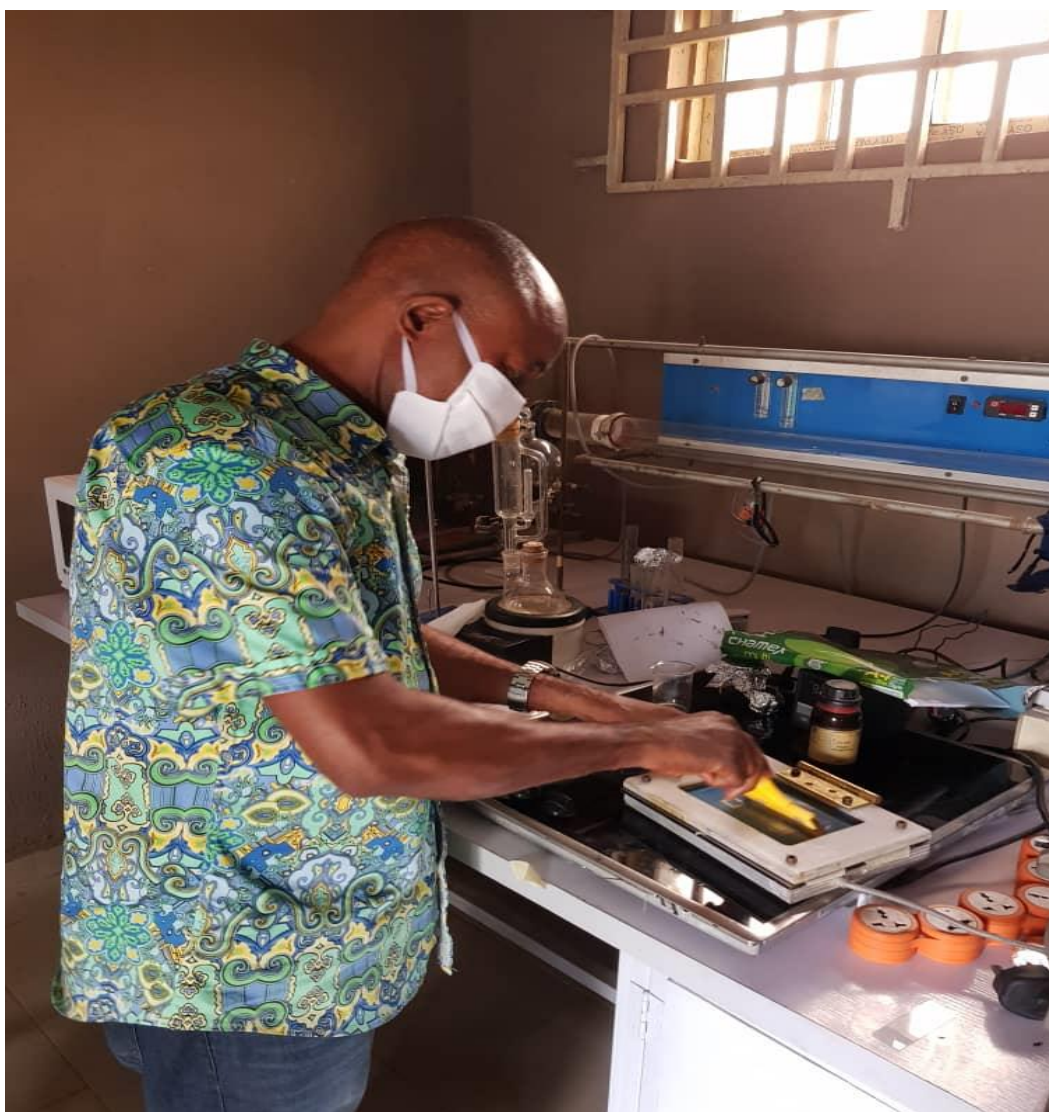
J: Screen Printing and Spin coating of \text{TiO}_2 -rGO
