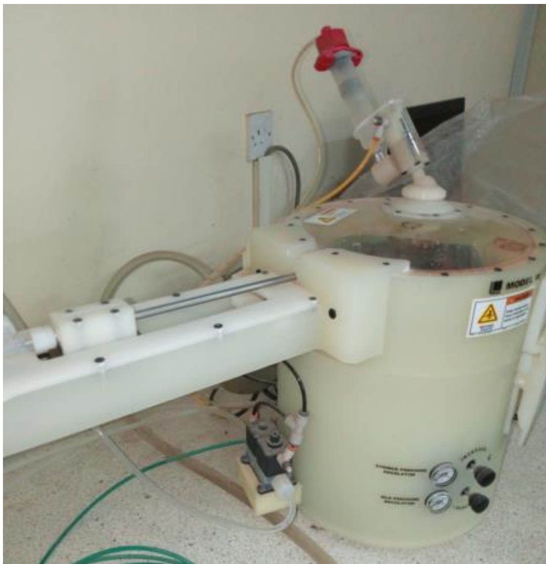
D: Spin-coater for deposition of the blocking layer (BL)
