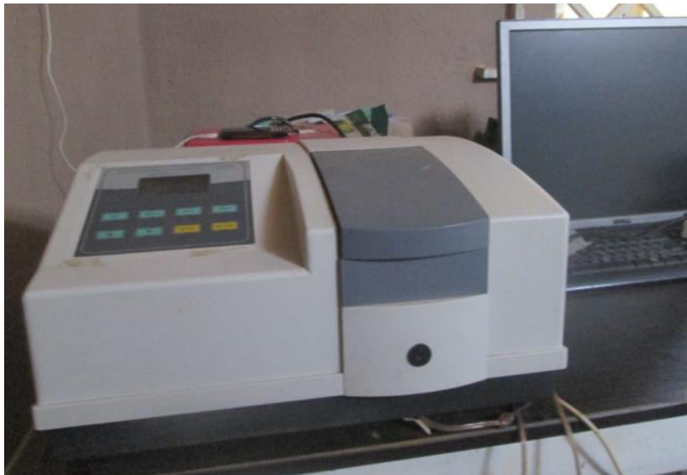
C: UV-Vis spec for photo-response determination
