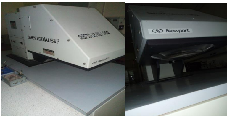
H: Solar Simulator for the determination of cell efficiency (I-V characteristics)
