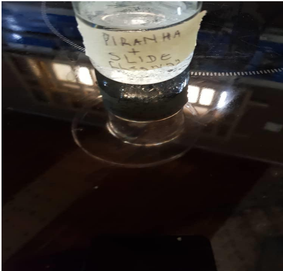
L: Piranha and slides (Cleaning of slides)
