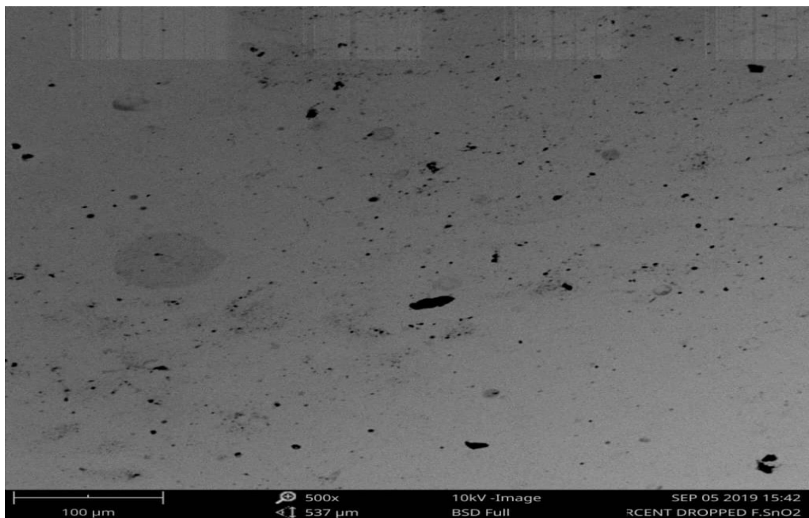
Figure 4.3: SEM of 8% F:SnO 2 with magnification size of 500x at 100μm
