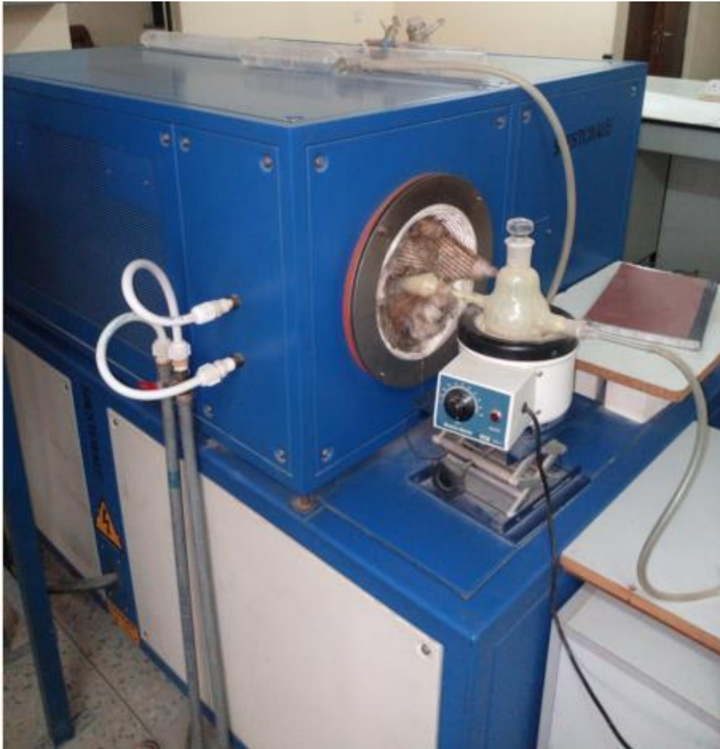
F: Furnace for annealing and sintering processes
