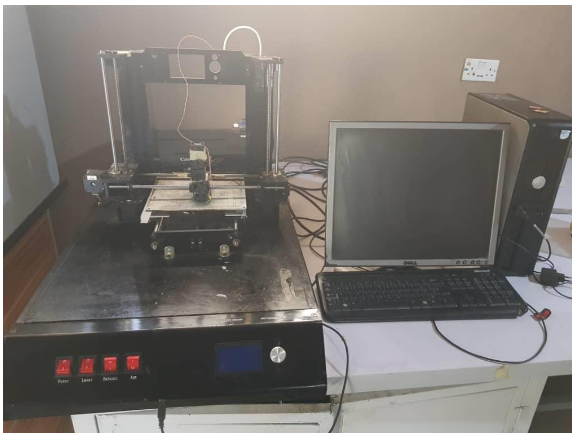
I: AACVD – Aerosol Assisted Chemical Vapour Deposition
