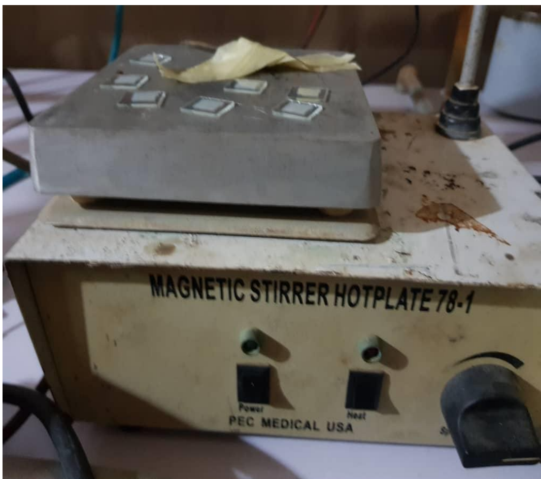
K: Magnetic Stirrer hotplate – drying of \text{TiO}_2 – rGO nano composite
