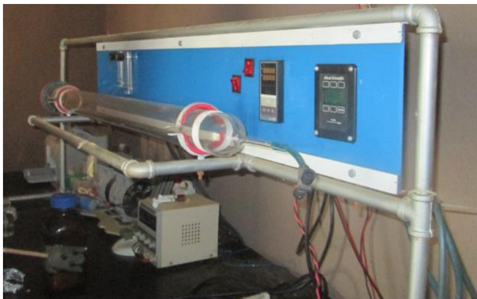
A: Chemical Vapour Deposition (CVD)
