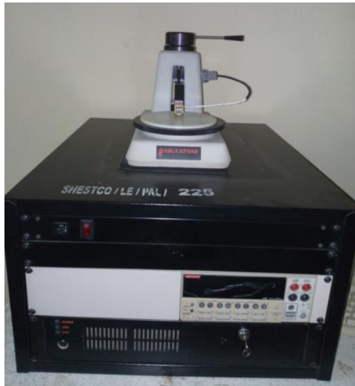
B : Four-point probe for electrical characterization
