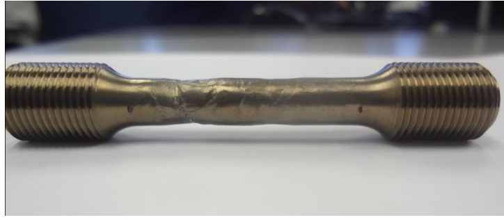
Figure 4.46: Exterior appearance of the titanium specimen after annealing and tensile testing, showing a slight discoloration
