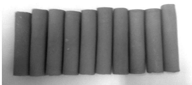
Figure 3.3: Titanium rods produced by cold isostatic pressing at a pressure of 700 MPa
