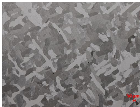
Figure 4.32: Microstructure of the titanium rods produced by cold isostatic pressing at 700 MPa followed by conventional sintering at 1350 °C for 1 hour
