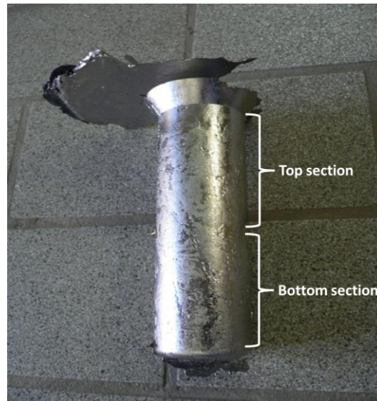
Figure 3.6: Cylindrical ingot obtained by vacuum casting of the cold isostatically pressed CP-Ti billet
