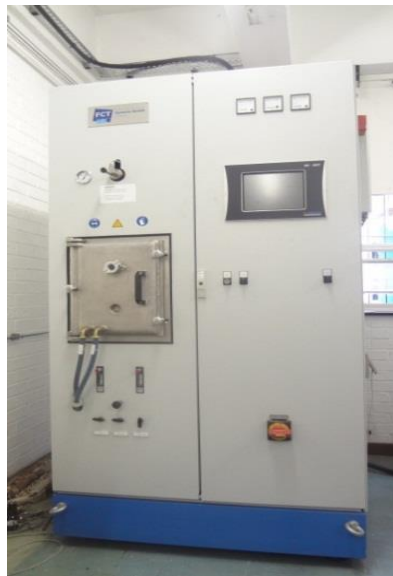
Figure 3.1: Spark plasma sintering (SPS) furnace
