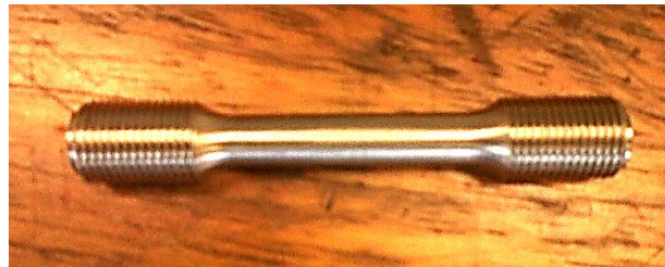
Figure 3.8: Cast titanium tensile specimen
