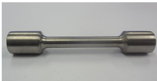
Figure 3.9: Exterior appearance of the fine polished Ti-6Al-4V specimen produced by rapid manufacturing
