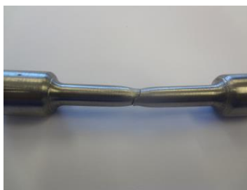
Figure 4.57: Pre-alloyed Ti-6Al-4V specimen showing a significant reduction in area and a cup and cone ductile fracture
