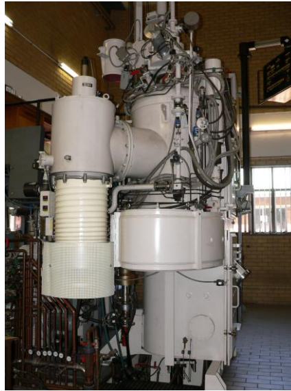
Figure 3.2: Leybold Heraeus ISPIII/Ds three chamber vacuum furnace
