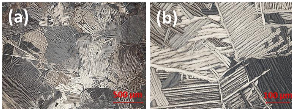
Figure 4.40: Optical microscopic structure of CP-Ti obtained by conventional casting in a vacuum chamber furnace at (a) low magnification and (b) higher magnification
