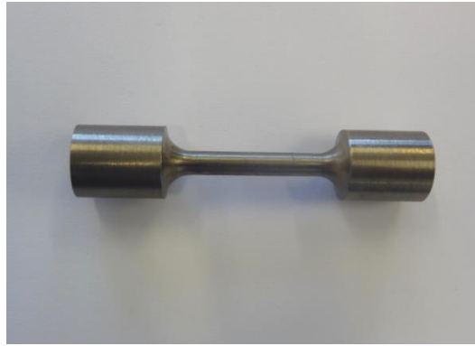
Figure 3.5: Exterior appearance of the tensile specimens machined from pressureless sintered titanium rod
