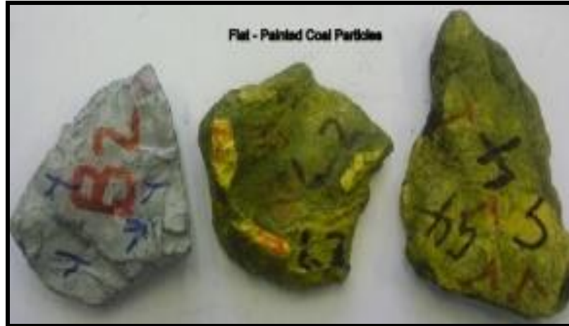
Figure 4.8(b): Flat Particles
