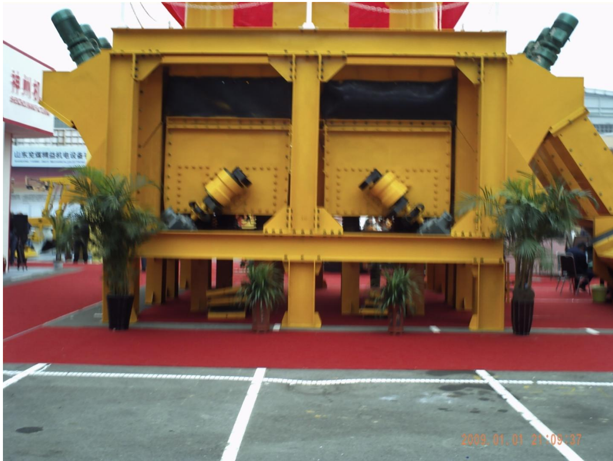
Figure 2.2: The 50ton/hr dry air dense separator in China
