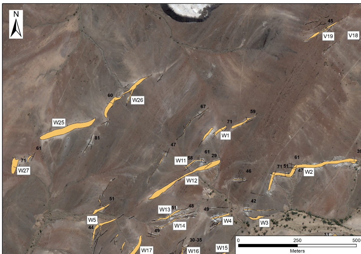
Figure 8: The northern portion of the Southern Cluster showing the location and extent of the W series pegmatites at surface.
