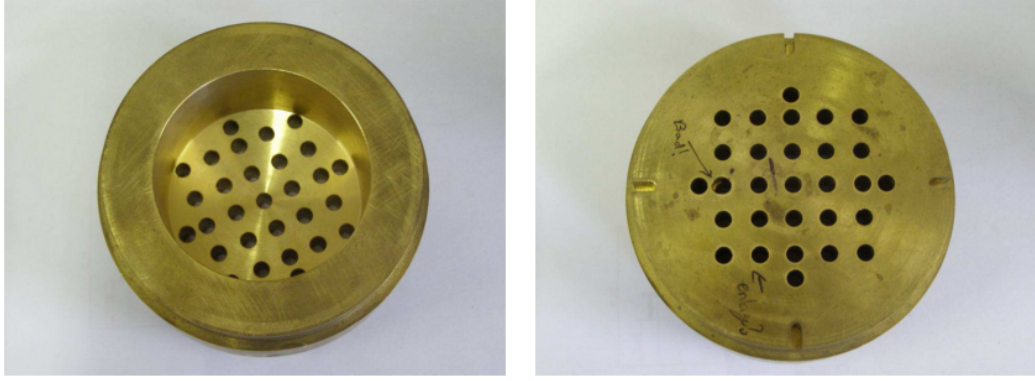
Figure 3.20: The pepperpot collimator used during experiments at iThemba LABS. The first hole relative to the middle of the collimator on the x -axis/ y -axis is centred at 0.819^\circ , the second at 1.679^\circ and the third at 2.251^\circ . These holes span 0.41^\circ .
