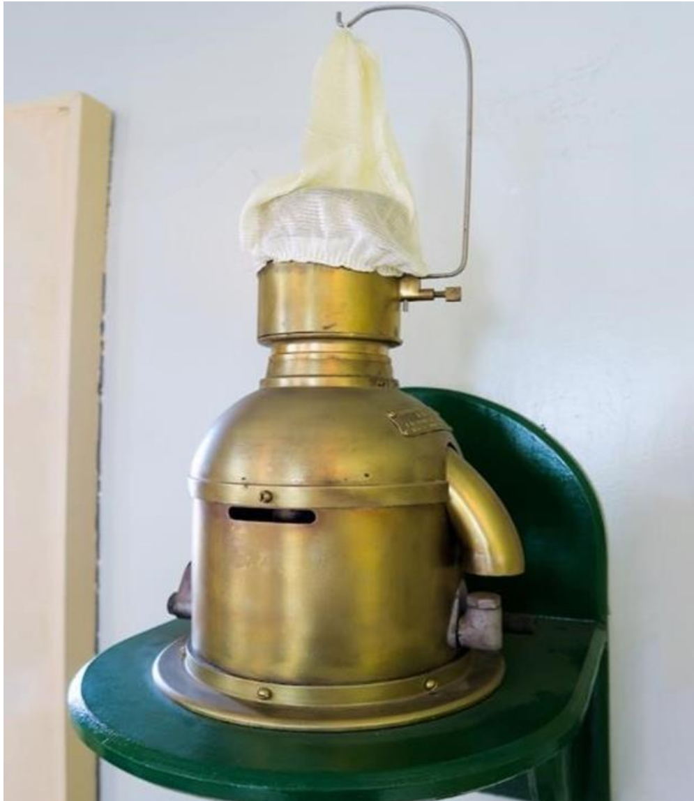
Figure 2. 2 Example of the petroleum vapour lamp with an unburnt mantle. Source (Etan J. Tal)
