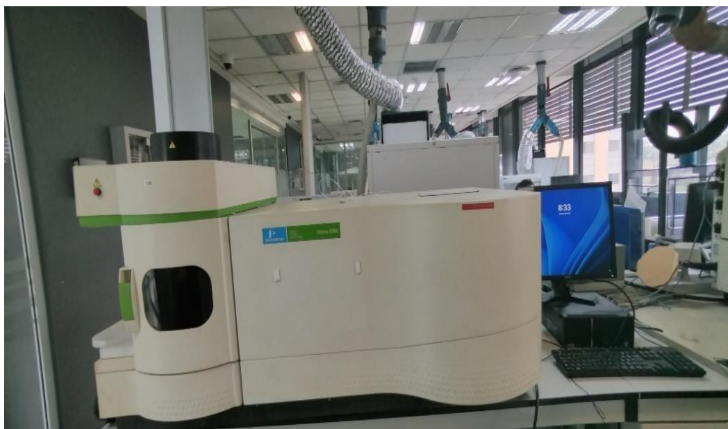
Figure 3.7 Inductively coupled plasma mass spectrometry (ICP-MS) Perkin Elmer 300Q NexION
