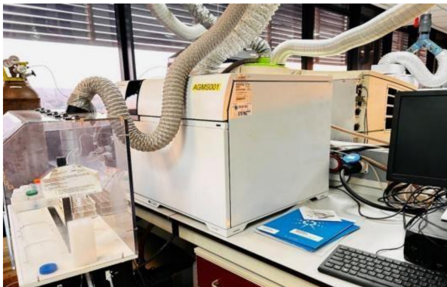
Figure 3.8 Inductively coupled plasma mass spectrometry (ICP-MS) Agilent ICP-MS 7800 instruments
