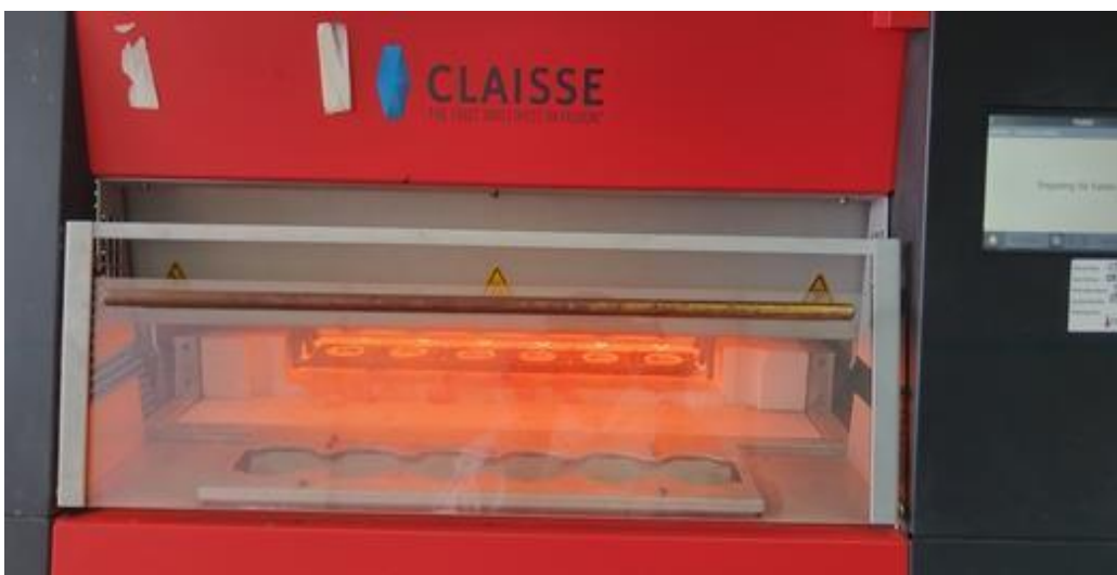
Figure 3.5 Samples placed in a pre-heated oven for efficient \text{LiBO}_2 fusion
