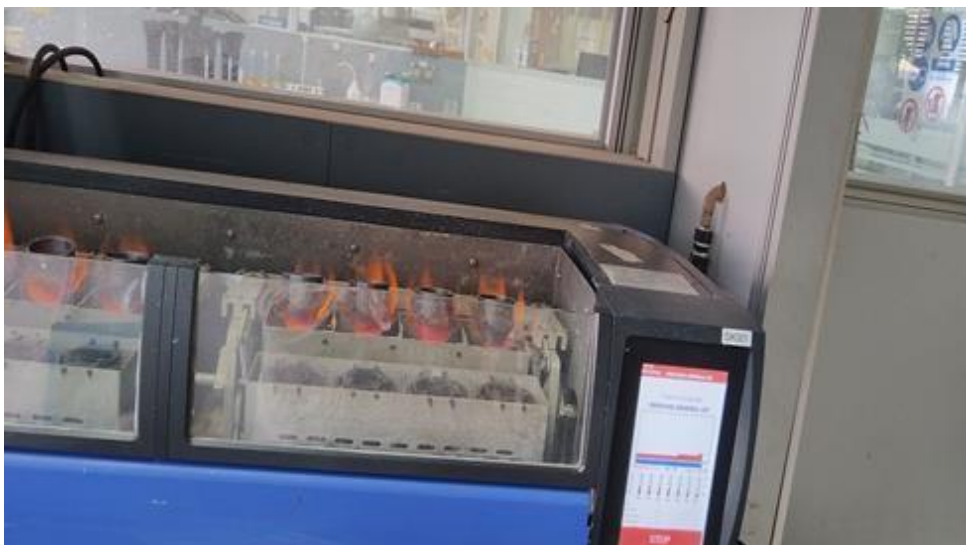
Figure 3.3 The sodium peroxide/ sodium hydroxide fusion in progress for the sample decomposition of the sample
