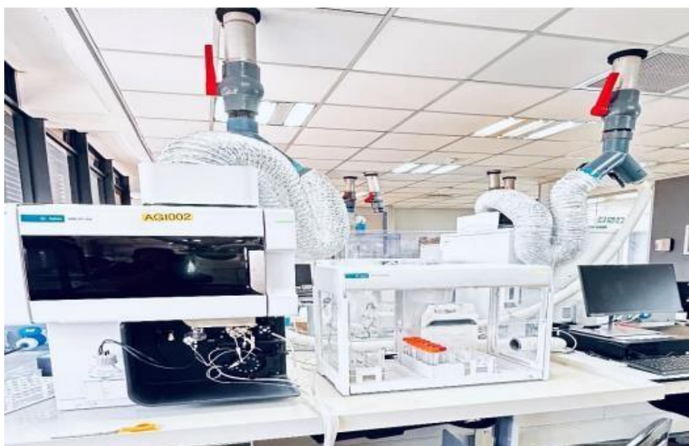
Figure 3.9 Inductively coupled plasma optical emission spectroscopy Agilent 5900 instrument for analysis of REEs
