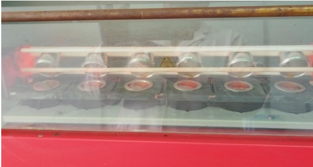
Figure 3.6 The completed cycle of LiBO 2 fusion with the homogenous melt casted on Pt mould
