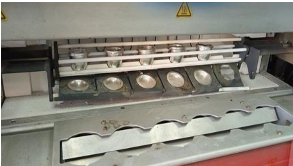
Figure 3 4 Mixture of samples and \text{LiBO}_2 flux placed on six position fusion machines
