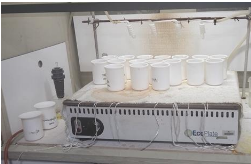
Figure 3.2 Hotplate assisted acid digestion using Teflon beakers
