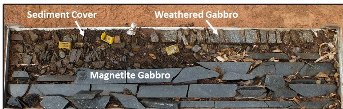
Figure 4.6. Unconsolidated alluvium and weathered sedimentary cover, as well as highly weathered gabbro overlying Magnetite Gabbro of the Upper Zone in core TW1.
