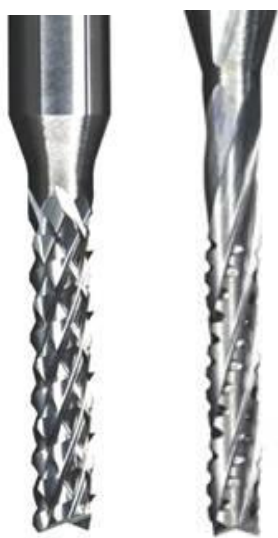
Figure 4.5: Teeth patterns of routers (a) diamond-patterned up cut, (b) spiral-patterned up-cut (Wulf, 2007)
