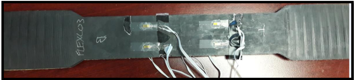
Figure 4-8: Belt sample with gauges attached.
