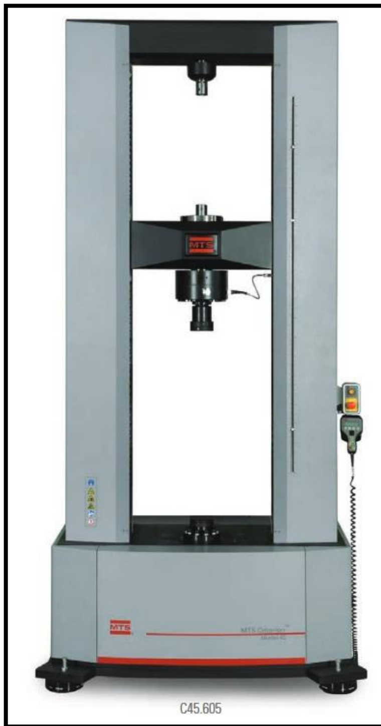
Figure 8-21: Illustration of an MTS Criterion C45 tensile tester.
