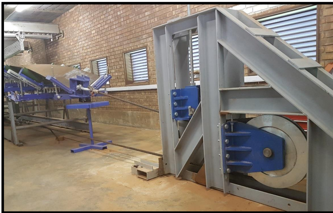
Figure 3-4: Image of the Sheave structure and belt attachment.
