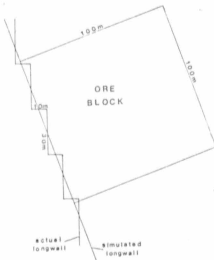
Figure 4.16a: Standard mining situation at time of ore block estimation, and simulated longwall position.
