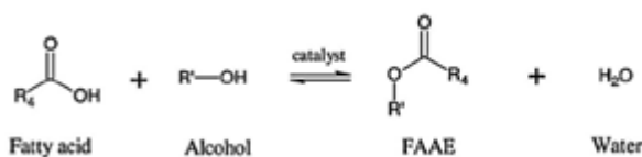
Figure 2.2: Esterification reaction of fatty acid with alcohol; \text{R}^4 is an acyl residue, \text{R}' is the alcohol moiety (Alaba, Sani and Ashri Wan Daud, 2016; Salam, Velasquez-Orta and Harvey, 2016; Lotti et al., 2018)
