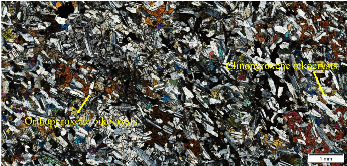
Fig. 6. 2. Microphotograph of the spectacular ophitic texture of the fine-grained Contact gabbronorite. It shows the plagioclase chadacrysts aligned subparallel. The orthopyroxene and clinopyroxene oikocryst optically encloses plagioclase chadacrysts.
