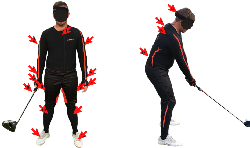
Figure 3.2: Figure showing the Xsens sensor locations
