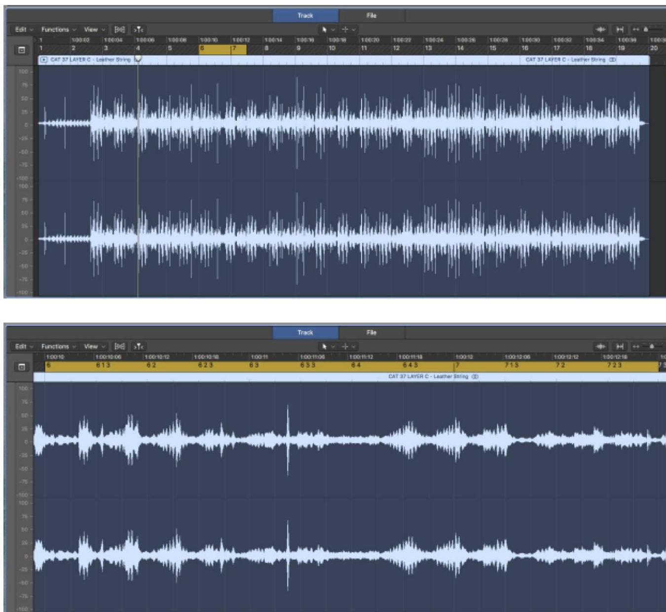
Fig. 8. Wave output of MR 37 replica, illustrating below in detail a section of the soundtrack above, highlighted in orange. The frequency output maximum measured 250 Hz using Logic Pro. (For interpretation of the references to color in this figure legend, the reader is referred to the web version of this article.)
