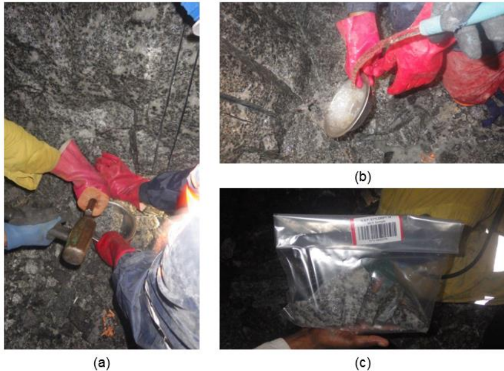
Figure 16. (a) Chipping of samples with a chisel from bottom to top of the sample channel; (b) Washing of sample instruments and bowl after every sample to prevent contamination; (c) Samples put into clean bags which are properly labelled.
