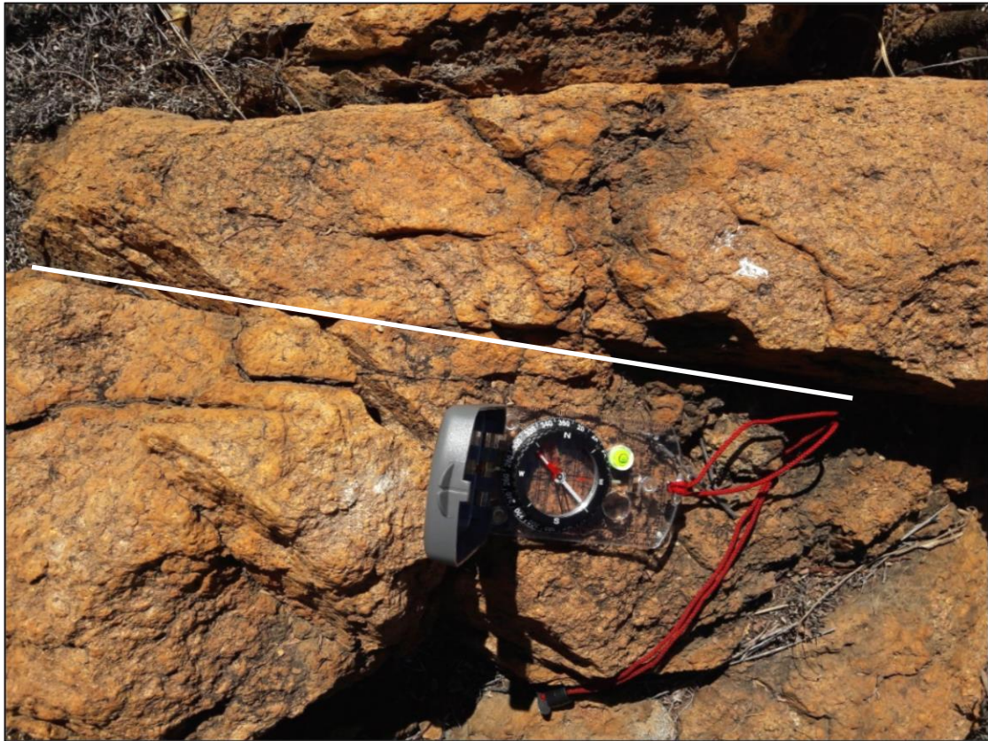
Figure 19. The 163^{\circ}/67^{\circ}\text{NE} conjugate fracture in the vicinity of the Roodekoppies Dam found on the highly weathered Lebowa Granites. The surface on the image is highly weathered, however, the fresh surface shows a pink to pale pink coarse-grained rock (granitic). The compass-clinometer represents the scale; the north arrow has deviated due to the uneven rock where the compass-clinometer is placed.
