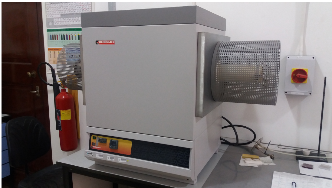
Figure 4.3: A photograph of a Carbolite high temperature horizontal thermal tube furnace. A wire wound tube furnace (CTF 17/300) with a 0^{\circ}\text{C} – 1700^{\circ}\text{C} temperature range.
