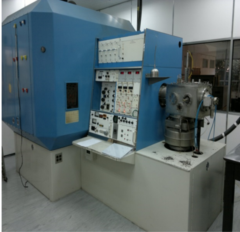
Figure 4.1: Photograph of the ion implanter at iThemba LABS. A Varian-Extrion model 200-20A2F.
