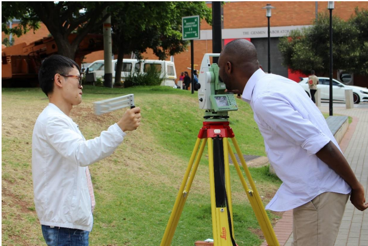
Figure A3: Survey of the Control Beacon from an existing Control points.
