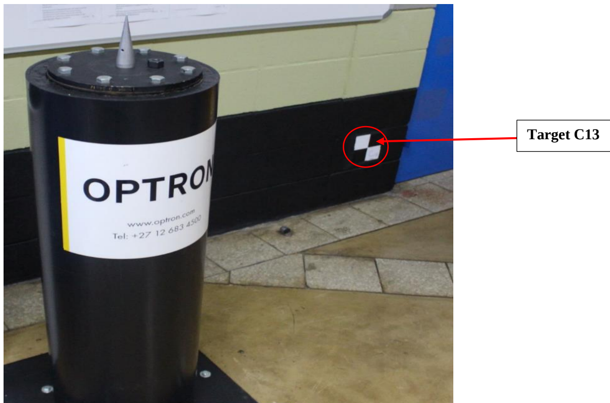
Figure 6.3: Illustration of Lower Vertical Angle between the Control Beacon and Target C13.
