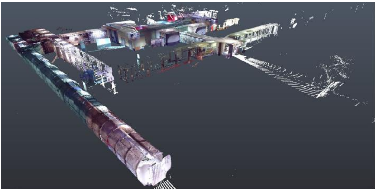
Figure 6.12: Showing Point Cloud Data View of the Chamber of Mines Building at the University of Witwatersrand.
