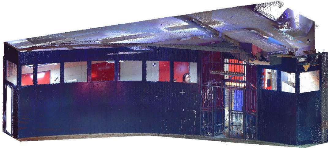
Figure 6.11: 3D Point Cloud of the Scanning Laboratory Imported to Cloud Compare with 27 Million Points.
