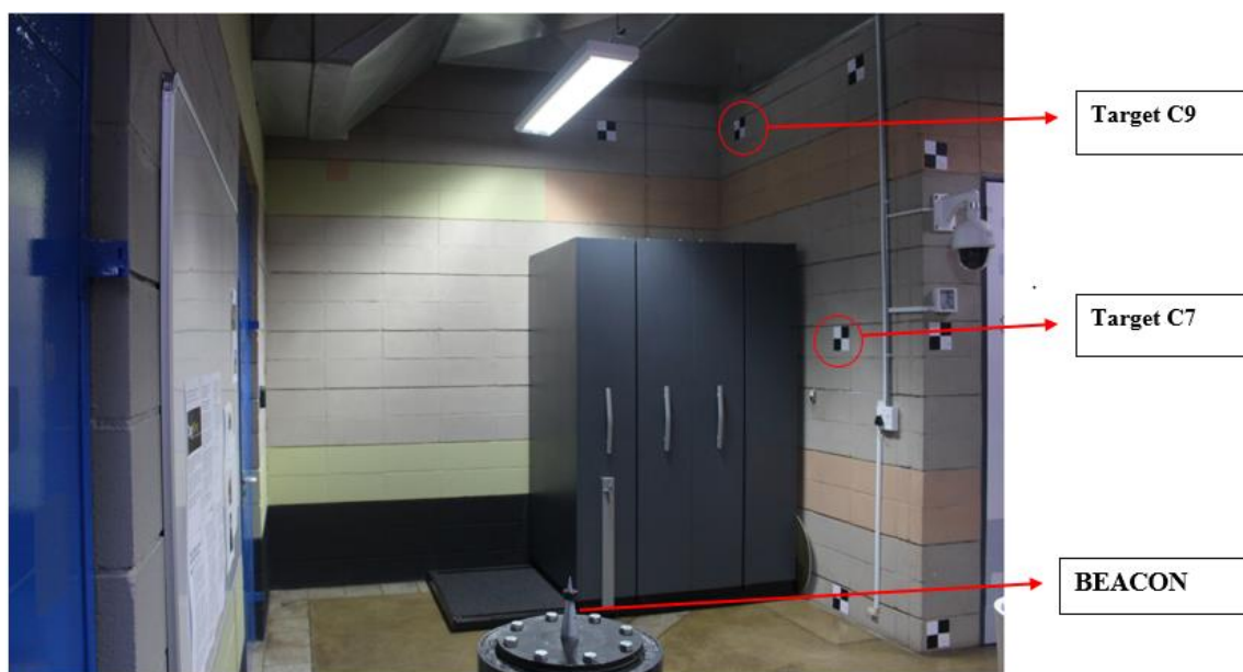
Figure 6.2: Illustration of Obliqueness of Targets C9 and C7.
