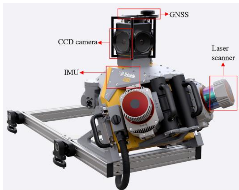
Figure 3.1: Image Showing Mobile Laser Scanner and Components (Ma, et al. , 2018)
