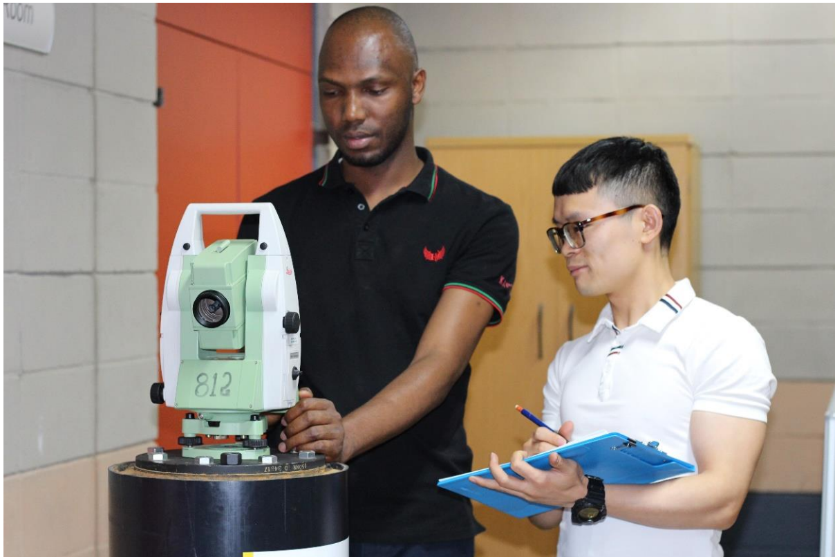
Figure A1: Setting up of Instrument on Control Beacon Coordinate
