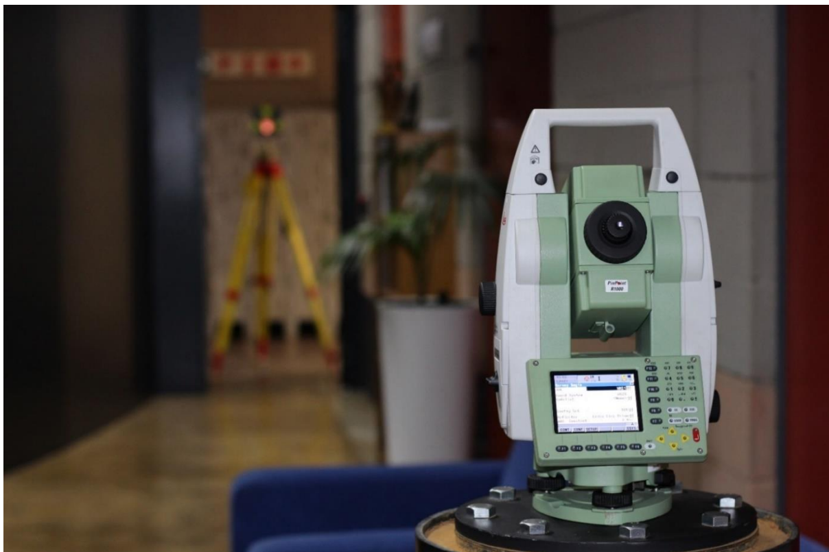
Figure A2: Survey of the Control Beacon with Leica Total Station
