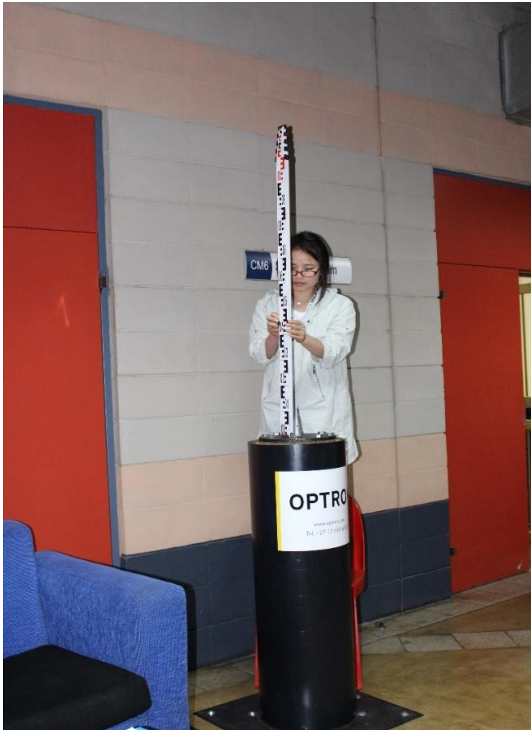
Figure B1: Levelling of the Control Beacon
