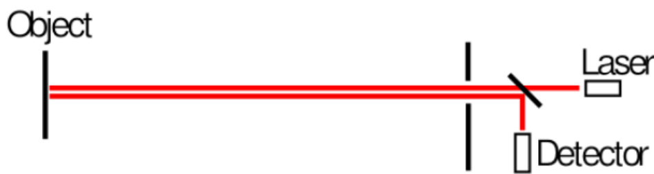
Figure 5.3: Theoretical Image of Time of Flight (Kaldén & Sternå, 2015)
