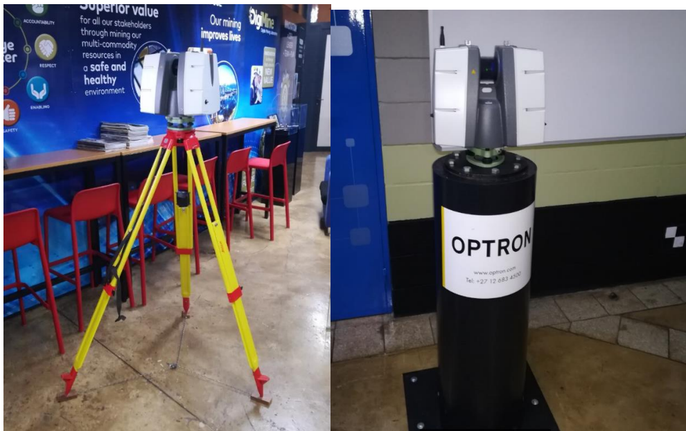
Figure 4.13: Photograph of the Terrestrial Laser Scanner Placed on the Control Beacon and Tripod Stand
