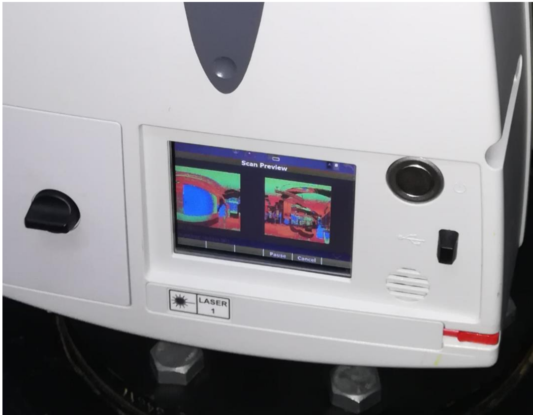
Figure E2: Preview of Scanned Surrounding from the TLS Mounted on Control Beacon
