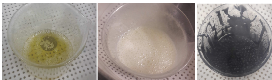
Figure 4-14: Images of bubbles being extracted in the samples after shearing, pure epoxy (left) BN/Epoxy (middle), C/Epoxy (right).
