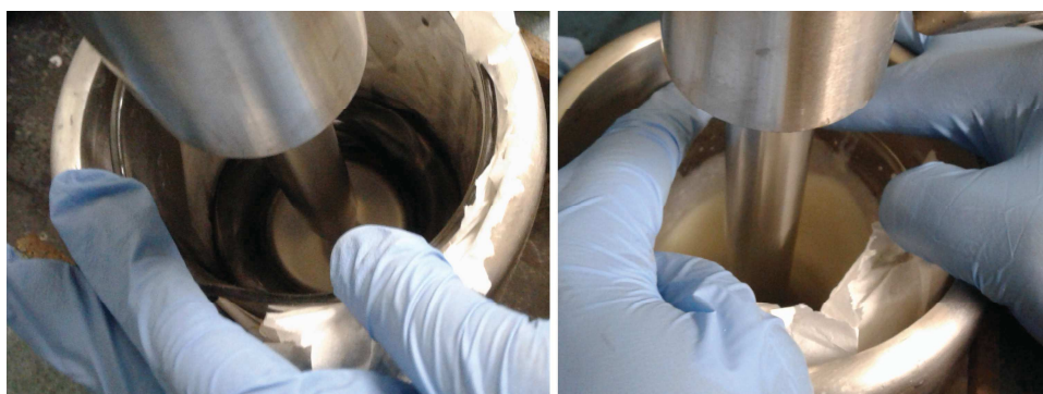
Figure 4-13: Image of C/Epoxy and BN/Epoxy during the shearing process.
