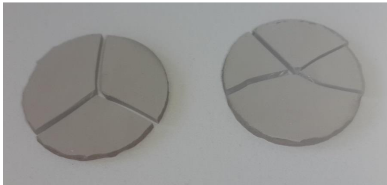
Figure 35: Typical mode of fracture observed showing initiation at the center of the samples.
