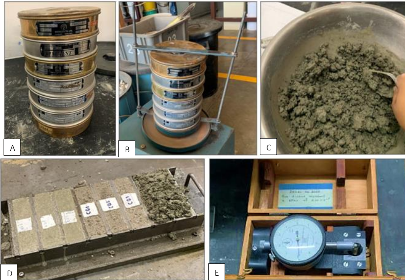
Figure 3.2: Images obtained from SANS 6245 methodology. A) Sieves used to grade aggregate with the opening from 4.75 mm, 2.36 mm, 1.18 mm, 600 \mu\text{m} , 300 \mu\text{m} , and 150 \mu\text{m} according to SANS 6245. B) Sieves on the shaker are used to adequately grade the aggregates. C) Cement, aggregate, and water mixed well to produce mortar. D) Compacted mortar with labels after tampering. E) Demec gauge instrument used to measure strain (with a factor of 2 \times 10^{-5} ).
