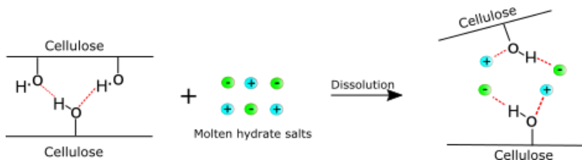
Figure 2.11 Dissolution mechanism of molten hydrate salts (Adapted from Fischer et al., 2003).
