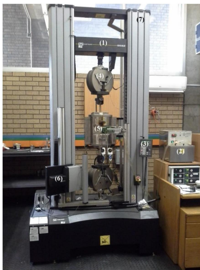
(1) Cross head, (2) Temperature controller, (3) Remote control (4) Clamp/Chunk with loadcell, (5) Heating furnace (6) Computer and (7) Test frame
