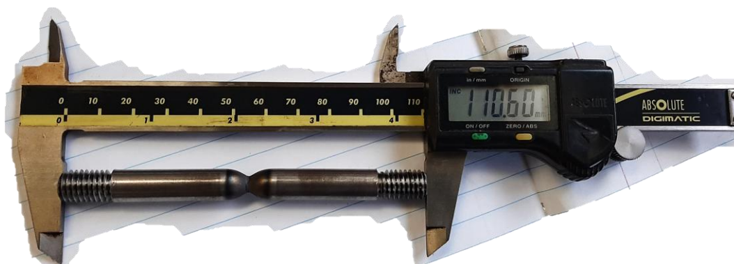
Figure 4.95 Typical post-test Gleeble® hot tensile specimen of the virgin parent material
