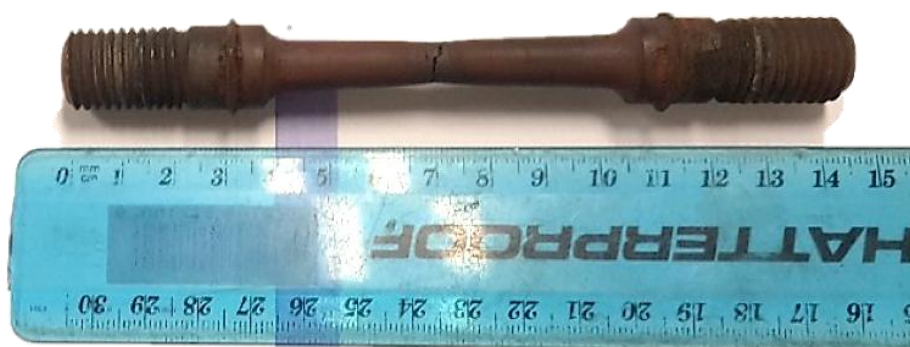
Figure 4.74 Ruptured creep specimen of the service-exposed parent material
