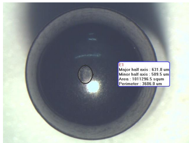
Figure 3.4 Measurement of the button wear area, A_b , of a WC-B button.
