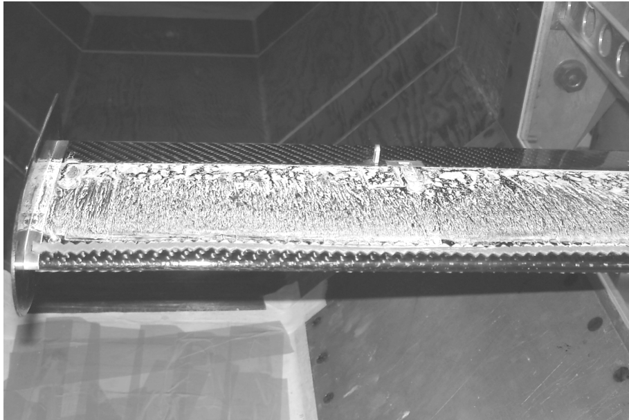
Figure 6.23 FAST Model Leading Edge Trip Strip and Attached Flow
