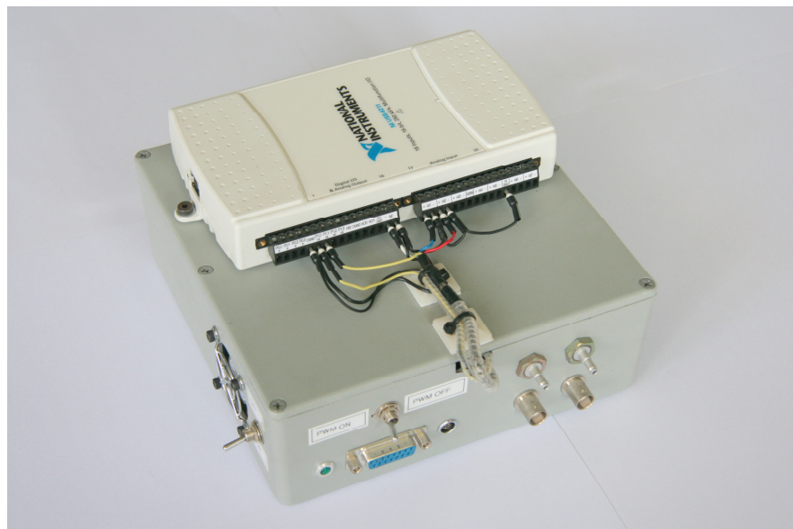
Figure 4.19 FAST Model NI USB-6211 DAQ and Instrumentation System
