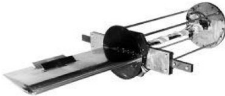
Figure 2.3 Pitch-Plunge Cantilevered Flexure Flutter Model (Waszak, 1997)
