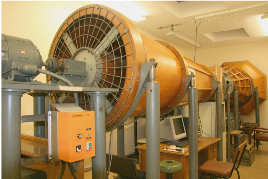
Figure 5.1 The CSIR's Calibration Wind Tunnel
