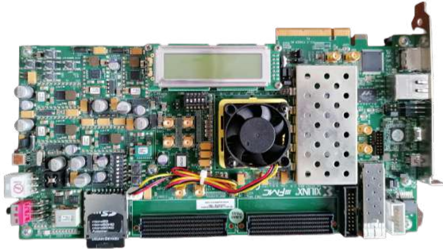
FIGURE 6.2: Xilinx VC707 evaluation board [115].
