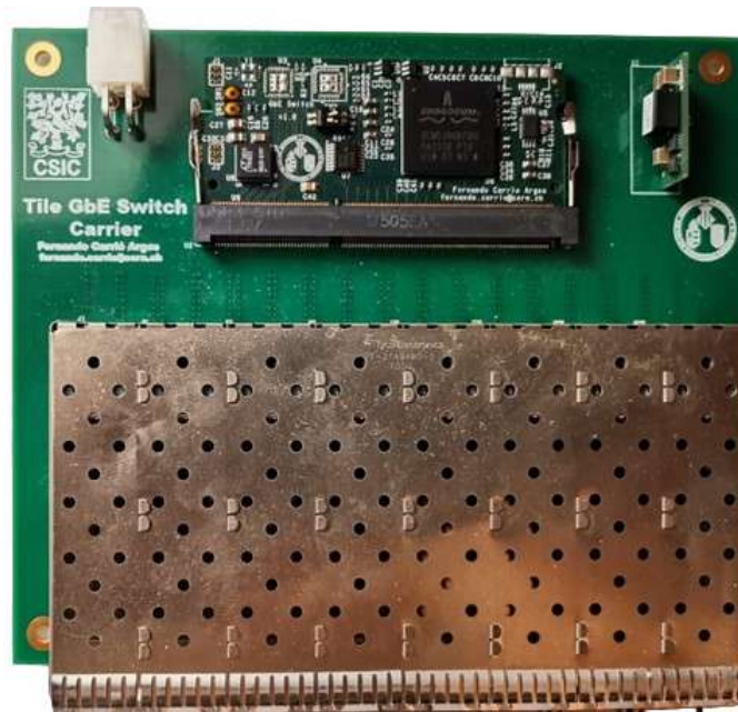
FIGURE 3.17: The Tile GbE Switch second prototype board produced in South Africa inserted in a motherboard.
