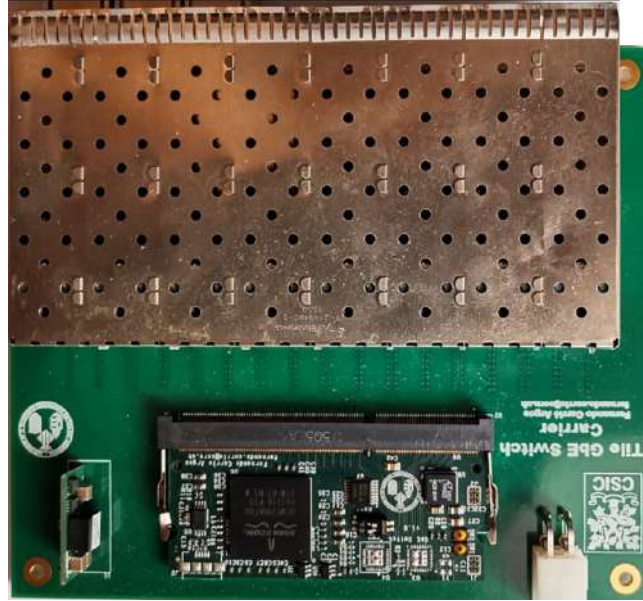
FIGURE 6.4: The Tile GbE Switch motherboard.
