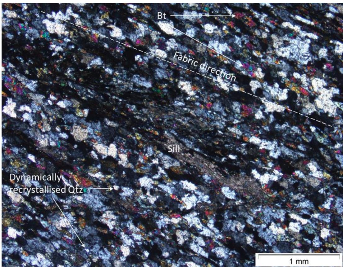
*Figure 3.14: Photomicrograph (XPL) of a mylonite sample collected near Camp I. The rock is predominantly fine-grained quartz, biotite and plagioclase. The rock is very fine grained and platy biotite and quartz are aligned in a strong fabric. Intense deformation has led to a grain size reduction through dynamic recrystallization, a texture typical of mylonite. Sample collected at GPS co-ordinates 28°0'6.58"N, 86°51'49.03"E.*
