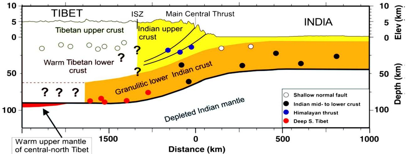
Figure 2.13: Granulitic lower crust subducted underneath Tibetan upper crust with limited downwards movement as its relative density is lower than that of the upper mantle. This results in a very thick crust approaching 100 km in thickness (after Jackson et al. 2008, from Dhital, 2015).
