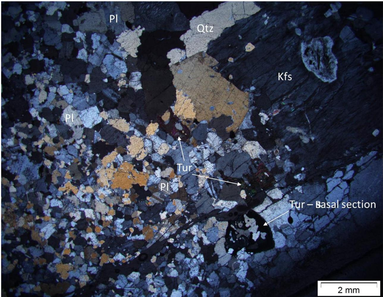
*Figure 3.7 Photomicrograph (XPL) of tourmaline granite. The rock is made up of quartz (Qtz), plagioclase (Pl) and K-feldspar (Kfs), tourmaline (Tur) and minor amounts of biotite. Some of the quartz is strained, indicating deformation after crystallisation of this granite. Sample collected at GPS co-ordinates 27°51'9.95"N, 86°51'4.30"E.*
