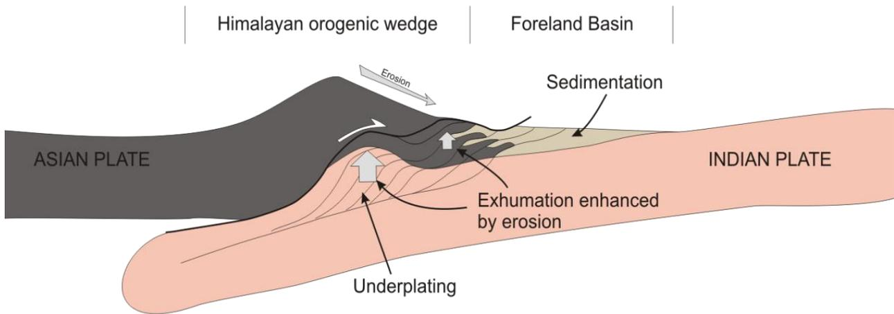
*Figure 2.14: Interaction between surface processes and exhumation in orogenic wedges. High rates of erosion allow underplated crust to be exhumed more rapidly along thrust planes (after Malavielle et al. 2008).*
