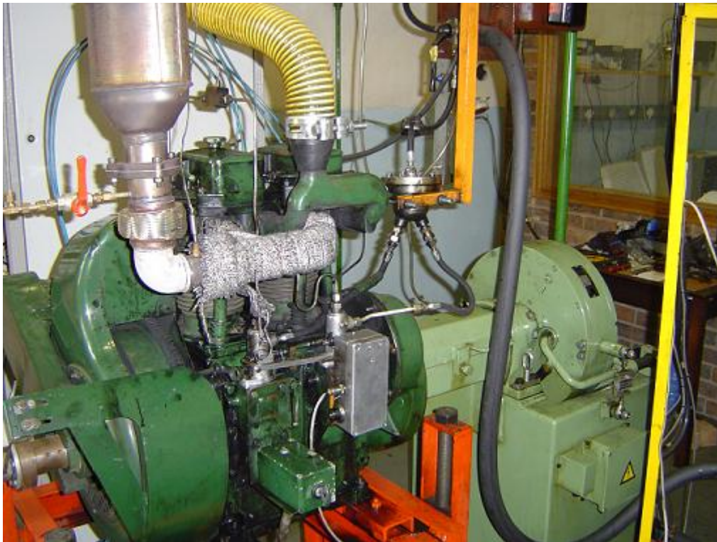
Figure 4.9 – Test engine with dynamometer
