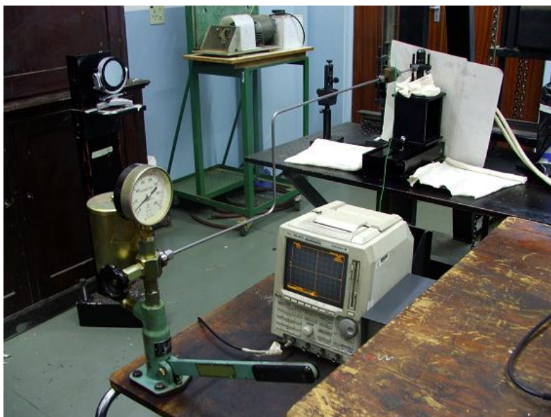
Figure 4.7 – Fuel Set-up with Diesel Reservoir
