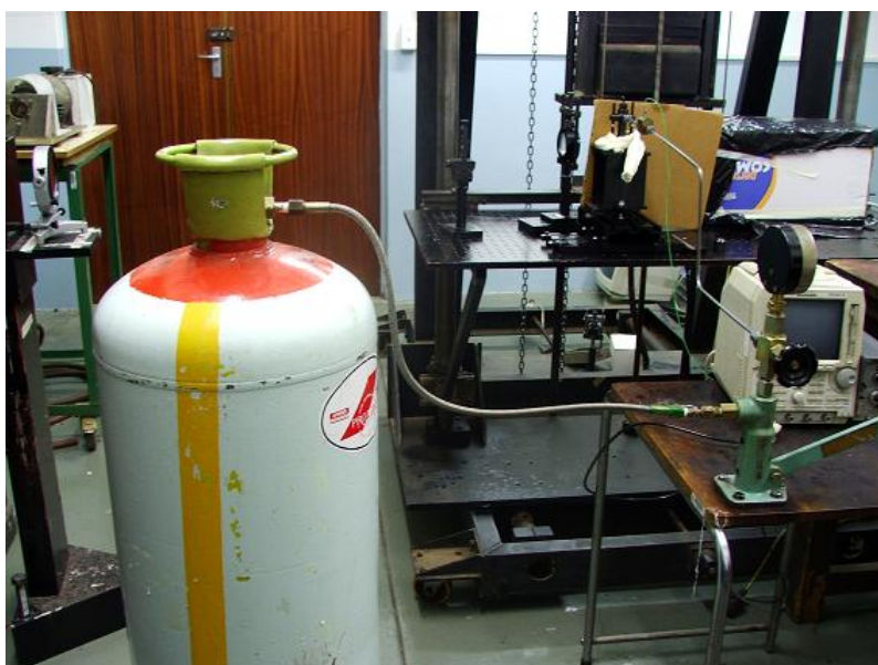
Figure 4.8 – Fuel Set-up with Dimethyl Ether Bottle Attached
