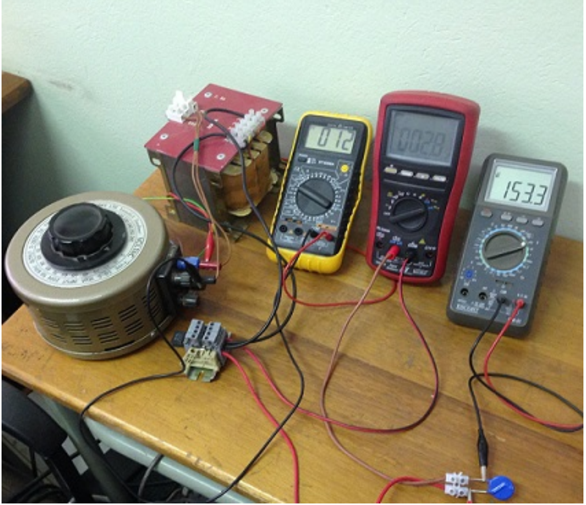
FIGURE 3.1: V-I test set up
