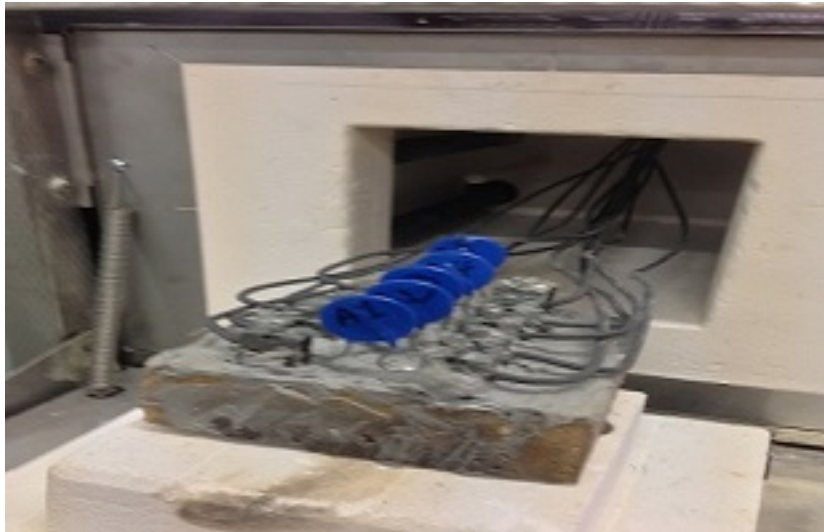
FIGURE 3.3: Connection arrangement of Varistor Samples
