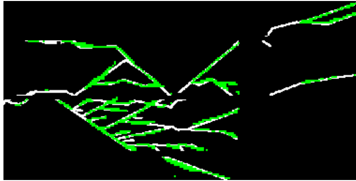
Figure 4.4: Crack layer for CFVS-00035-r8-c4 showing the prediction for cracks from the U-Net model (green) and the underlying ground truth mask (white). The IoU metric provides a numerical estimate of the overlap between the two.
