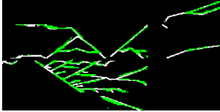
Figure 5.18: Crack layer for CFVS-00035-r8-c4 showing the prediction from the U-Net model (green) and the underlying ground truth mask manually coloured (white).
