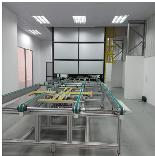
Figure 2.5: Example of an I-V and EL characterisation station typical of a PV module manufacturer
