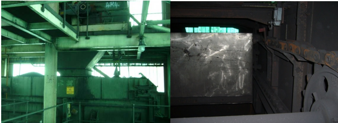
Figure 4: Illustrating the conveyor falling stream mechanical sampler and mechanism.
