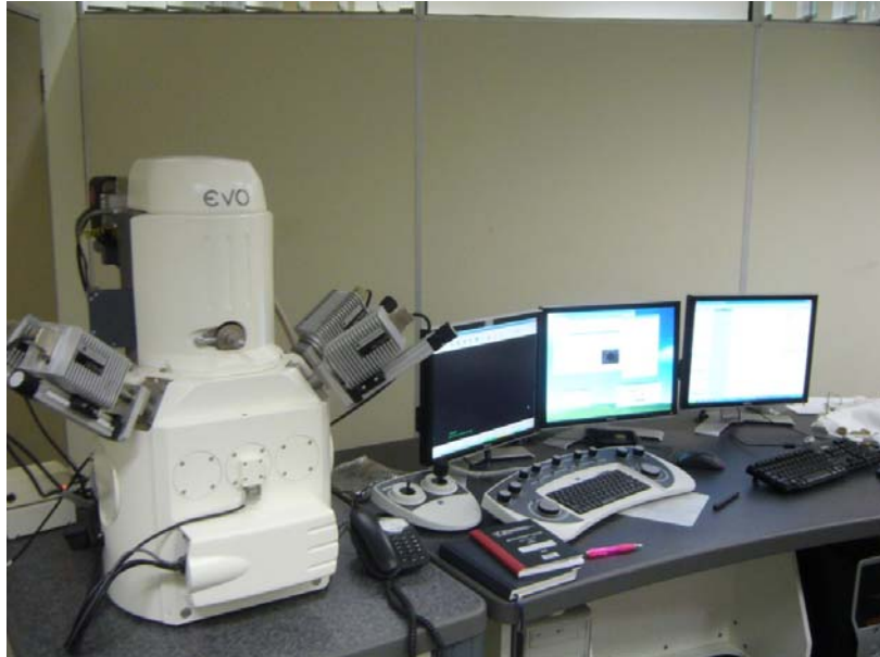
Figure 10: The QEM SCAN microscope used at ESKOM Research and Development for the mineralogical investigations.
