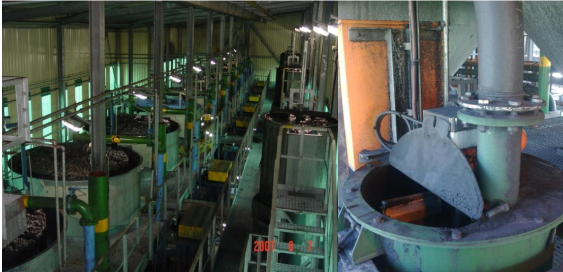
Figure 6: An illustration of the flotation plant and mechanical slurry stream samplers with which the samples were taken. The plant consists of three modules of three sets of primary and secondary cells each.
