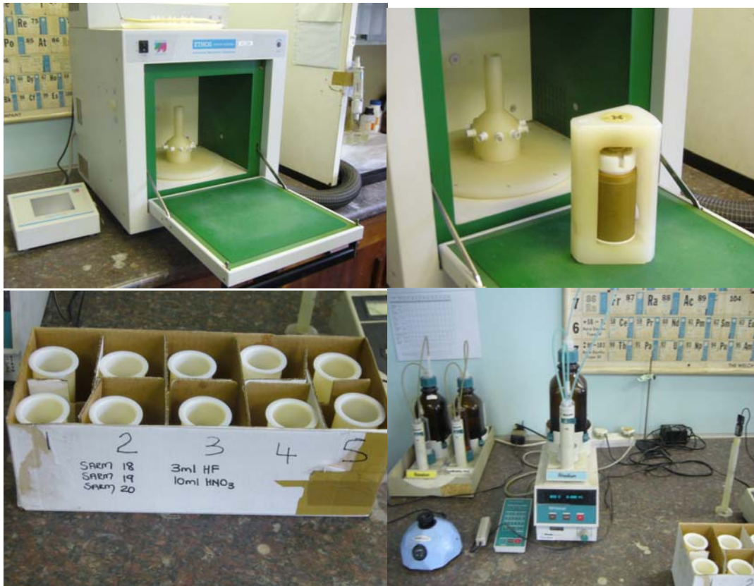
Figure 12: Illustrating the microwave digestion experimental setup.
