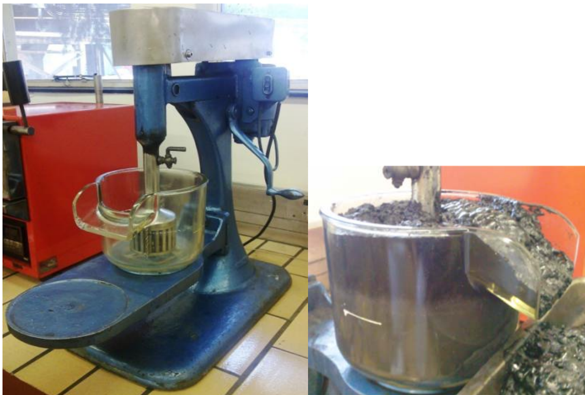
Figure 9: An illustration of the Denver flotation cell utilised to do the bench scale flotation tests.
