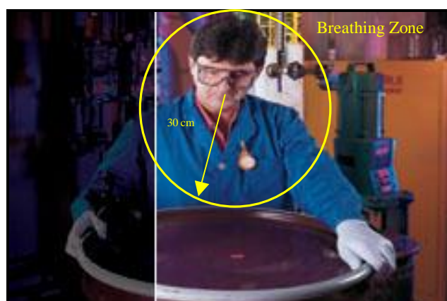
Figure 4: Typical placement of a Sample in a Worker’s Breathing Zone
