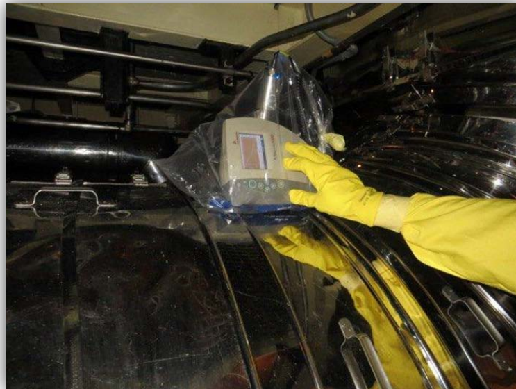
Figure 6.5: Measurement at Point 1 using Inspector 1000
