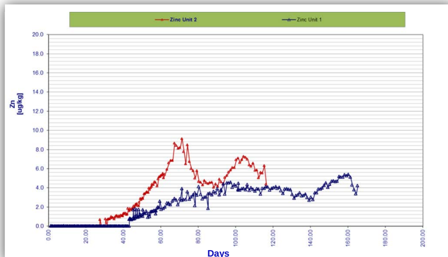
Figure 6.4: Zn measurements since initial injection (Koeberg Unit 1 and Unit 2)
