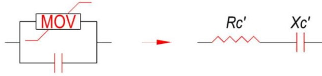
Figure 2-22: Linear approximation of and MOV protected series capacitor
