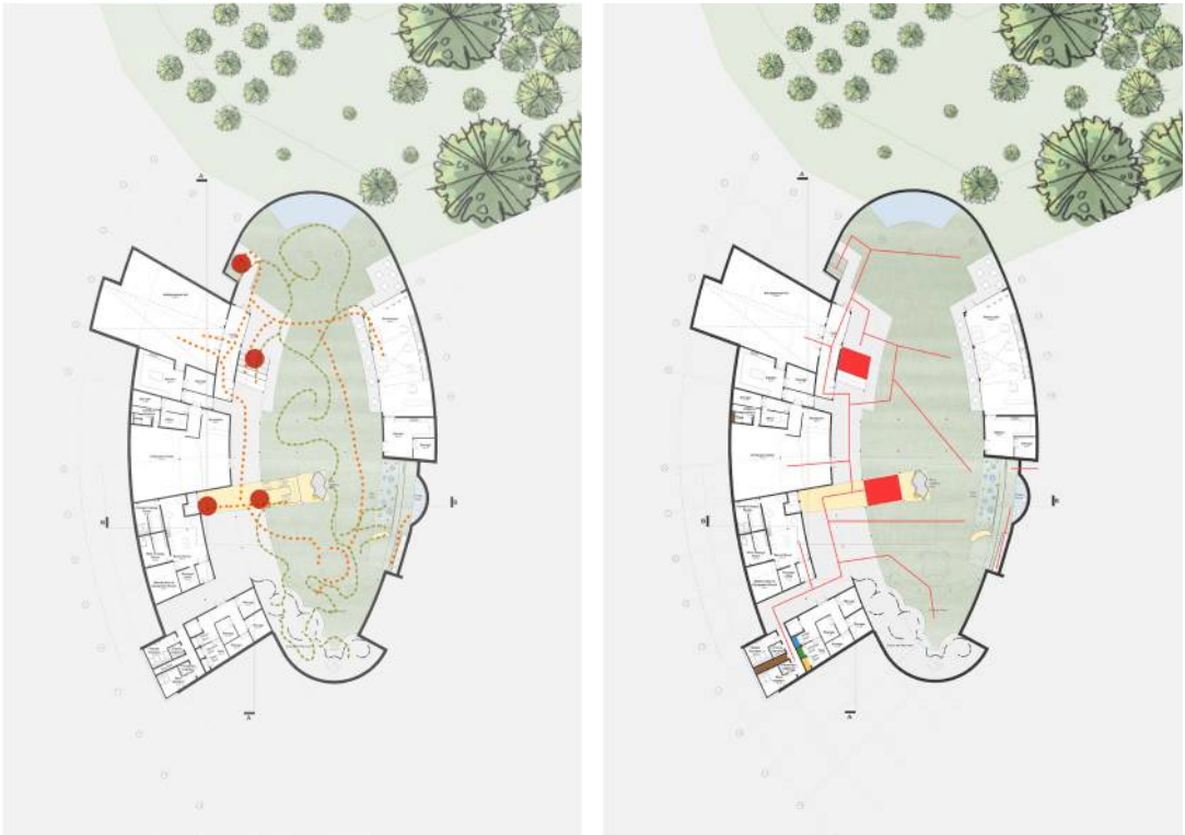
Figure 11.12: Access Points and Circulation (Author, 2024) Figure 11.13: Services and Escape Routes (Author, 2024)
