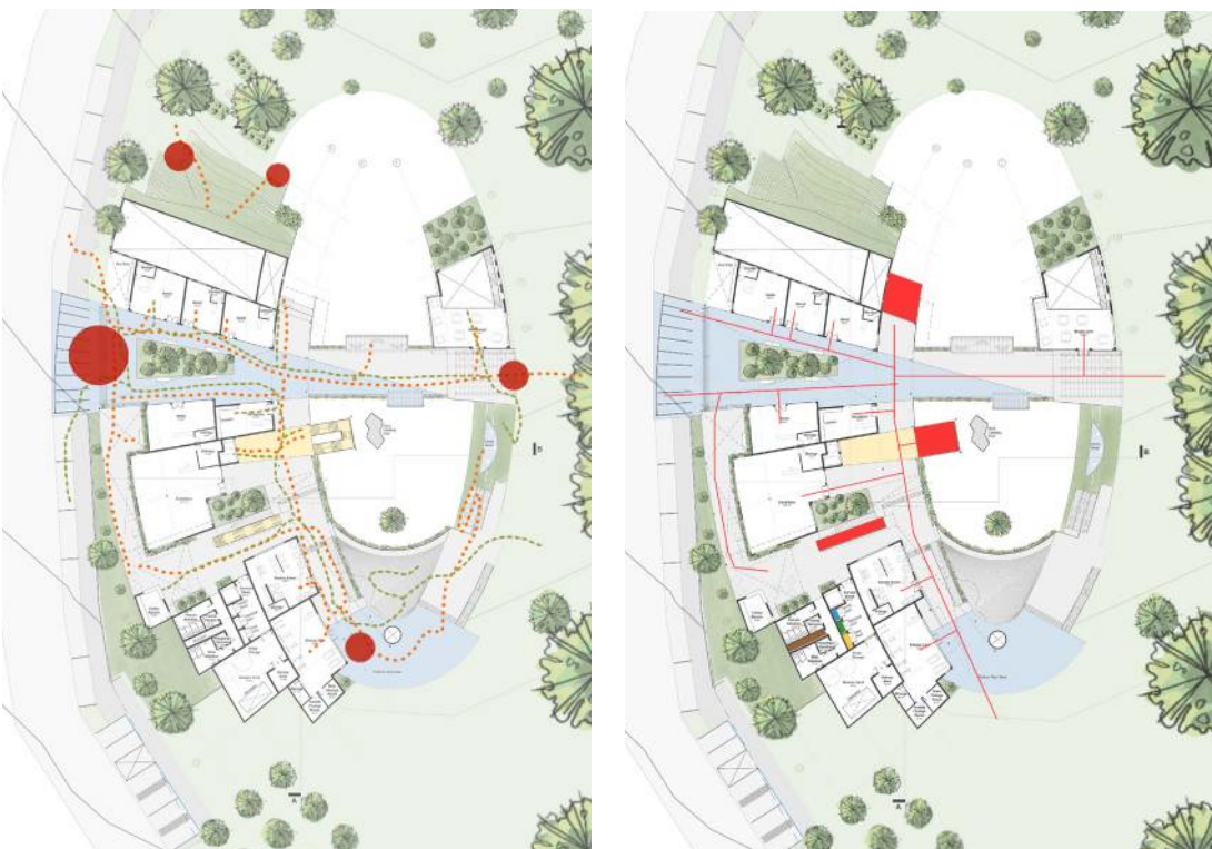
Figure 11.15: Access Points and Circulation (Author, 2024) Figure 11.16: Services and Escape Routes (Author, 2024)
