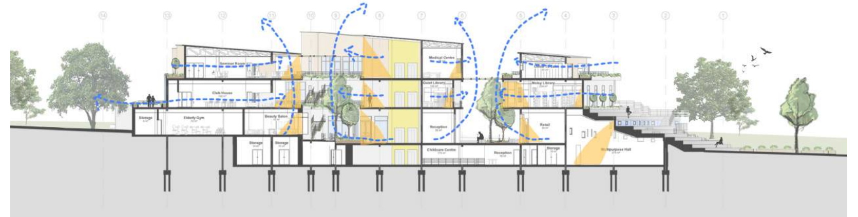
Figure 11.37: Diagram showing natural lighting and ventilation in Section A-A (Author, 2024)
