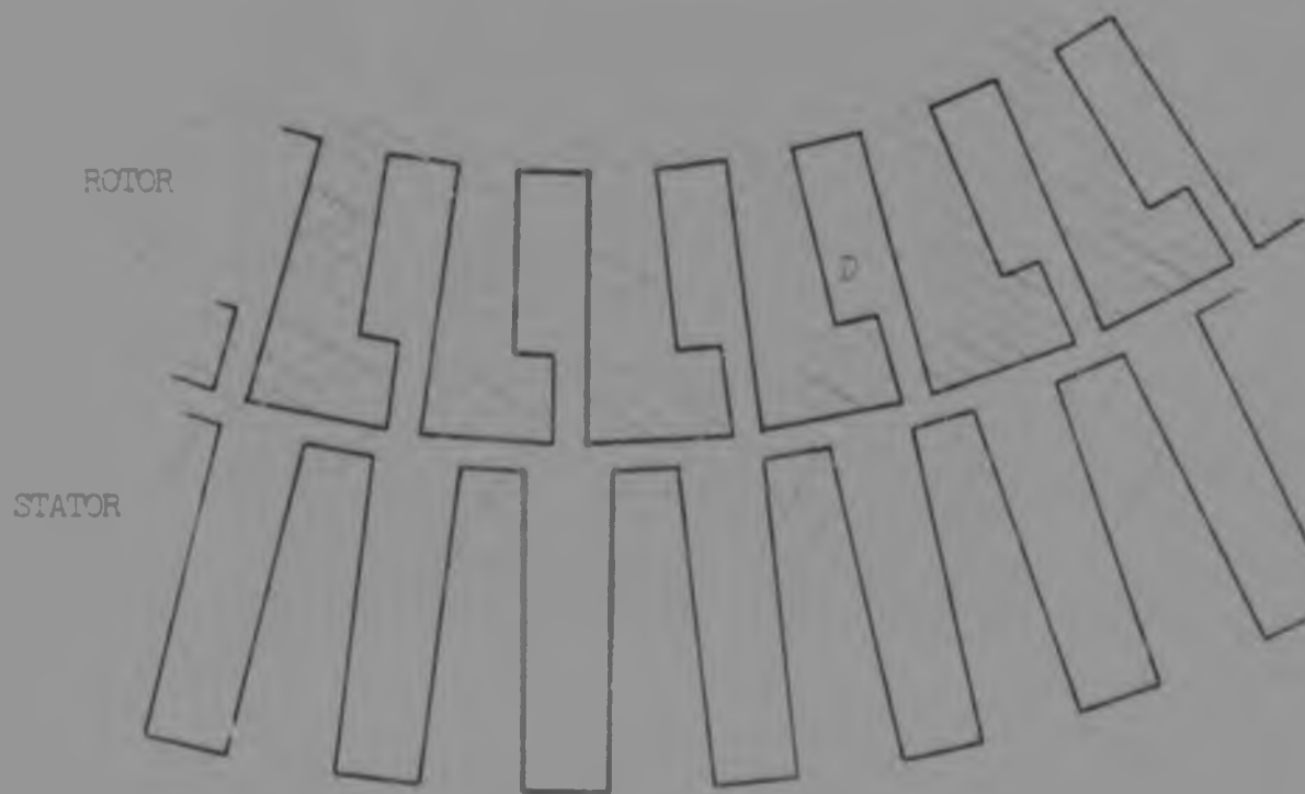
Figure D.6 - Relative position between stator and rotor teeth in industrial motor A during the bar current measurements.
