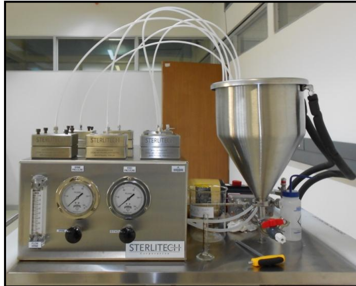
Fig. 3.4: Cross-flow filtration system used in this work.
