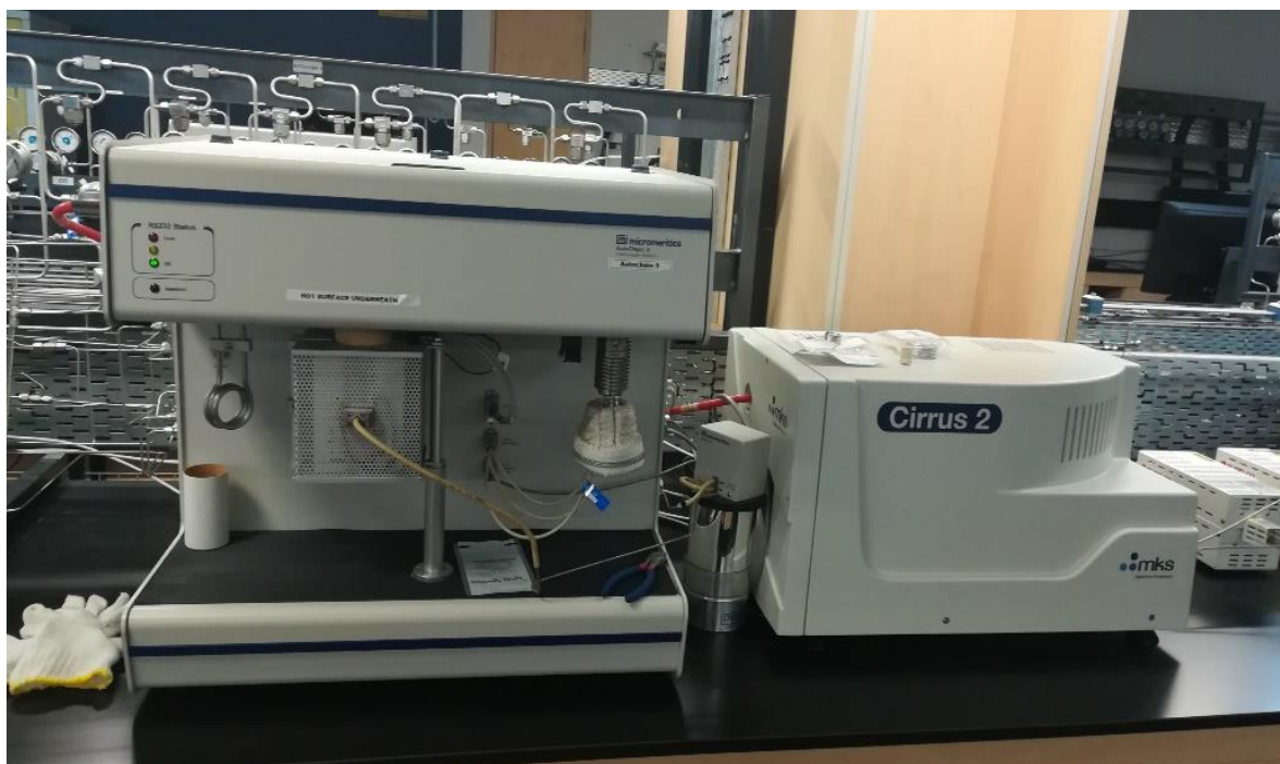
Figure 3. 4 AutoChem 2920 (Micromeritics, USA coupled to a Cirrus Mass Spectrometer (MKS Instruments)
