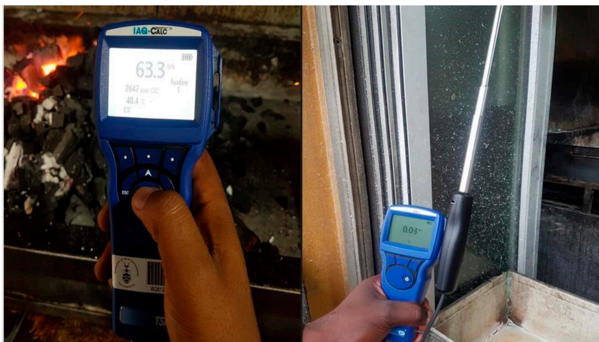
Figure 5. Q-Trak I IAQ meter for monitoring temperature, humidity, CO, and CO 2 (TSI Inc., Shoreview, USA).
