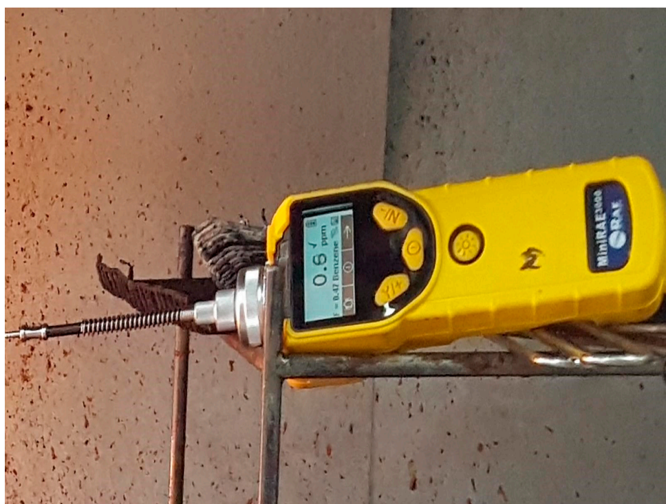
Figure 4. Photoionization detector (PID), MiniRae 3000 (RAE Systems, Inc., Kent, WA, USA).
