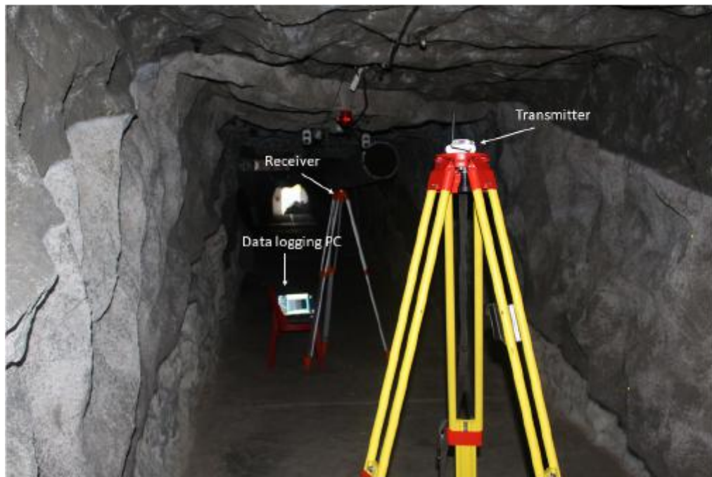
Figure 5.1: Transmitter node, receiver node and data logging computer used for performance measurements.
