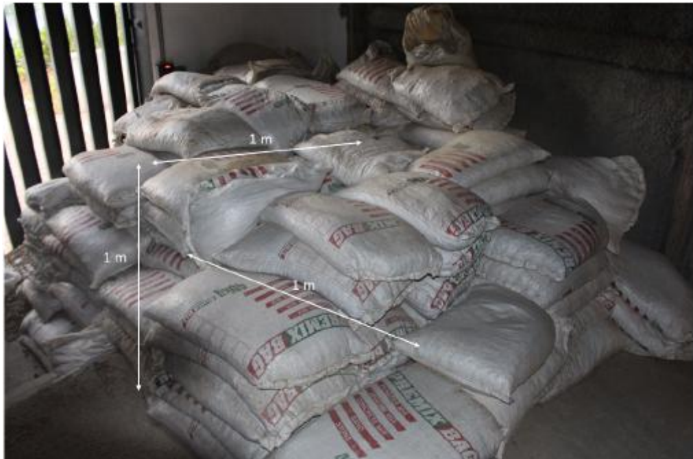
Figure 5.3: Collapsed scenario with the transmitting node buried underneath the rubble (dimensions depicted are approximately 1m in dimensions).
