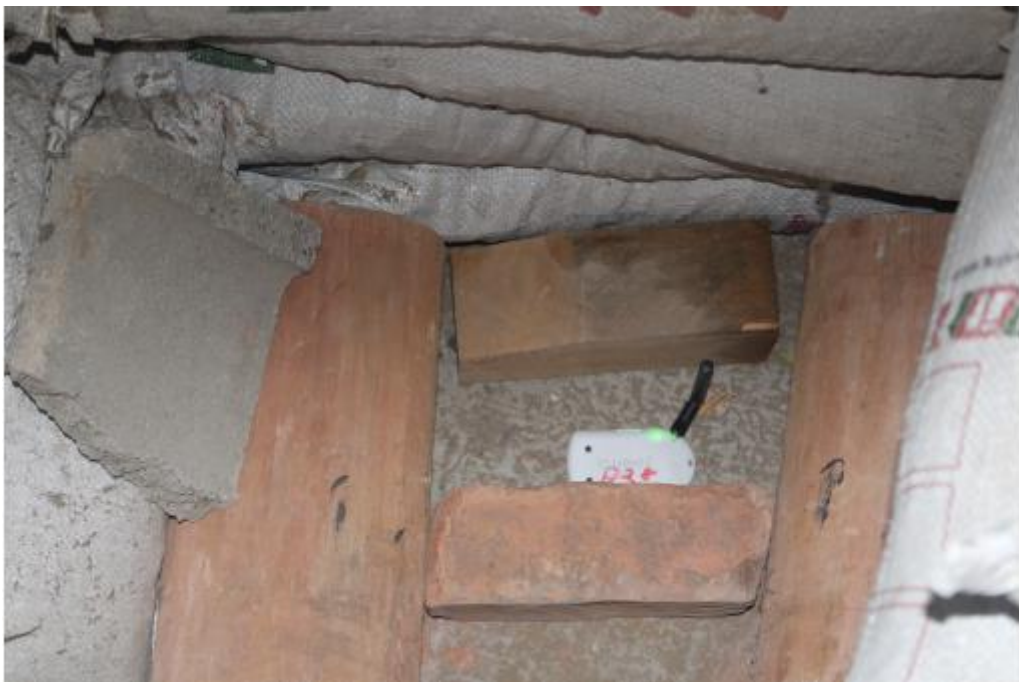
Figure 5.6: Collapsed scenario showing a closer look at the transmitting node at the bottom of the rubble before burial.
