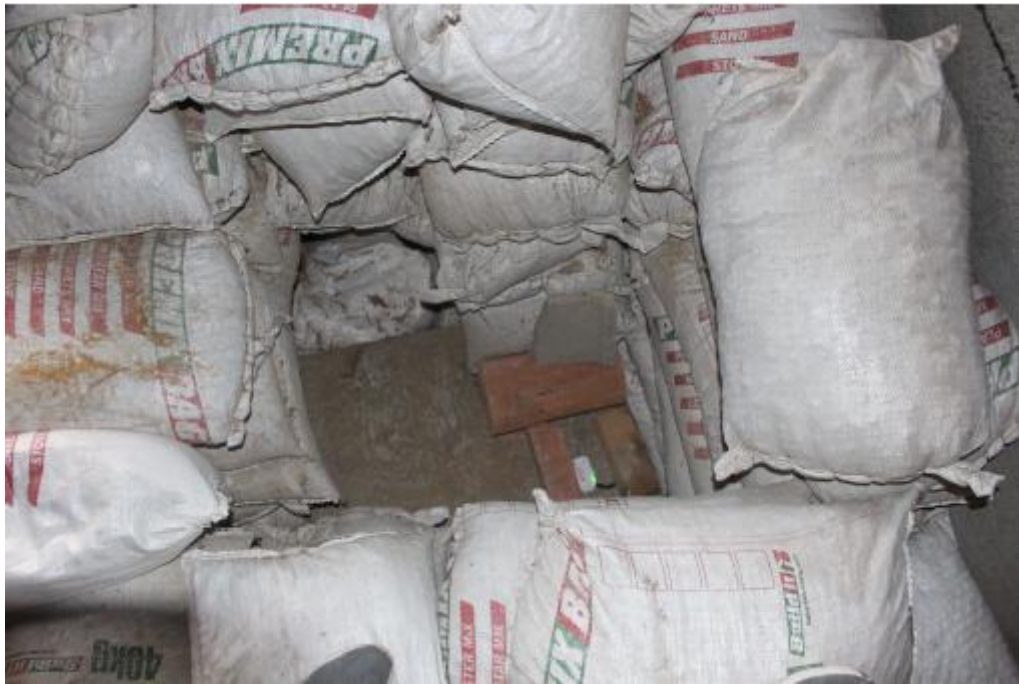
Figure 5.5: Collapsed scenario showing the transmitting node at the bottom of the rubble before burial.
