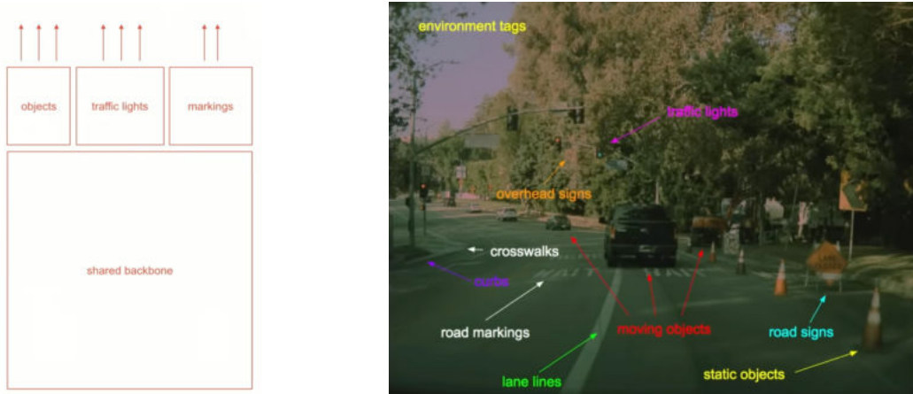
(a) Shared backbone architecture (b) An example RGB scene with extracted labels
