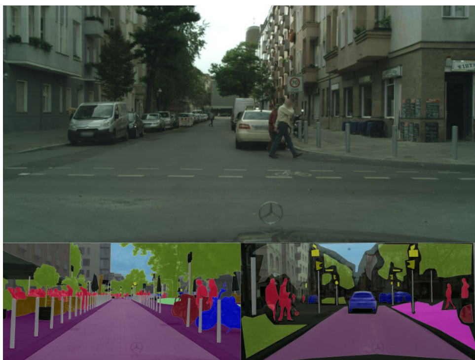
Figure 2.15: Example data from The Cityscapes Dataset. The top image is a blurred example RGB frame from the Berlin sub-set. The bottom left image is an example of a fine segmentation map from Stuttgart, and the bottom right is an example of a coarse segmentation map from Nuremberg [Cordts et al. 2016]
