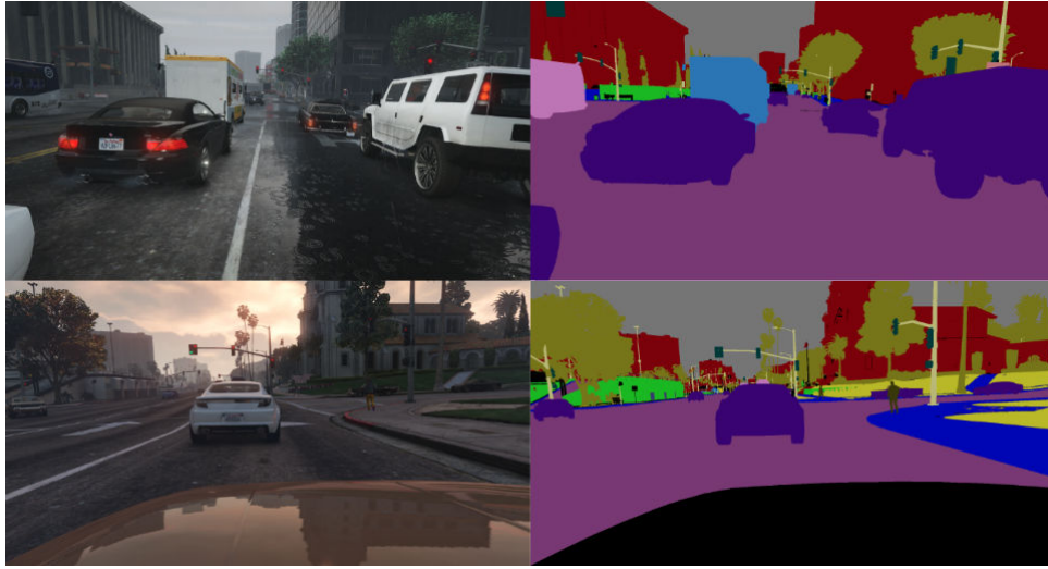
Figure 2.16: Example data from the From Games dataset. The left side represents two front facing image samples from the dataset, with the corresponding segmentation label on the right [Richter et al. 2016b]
