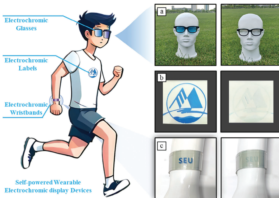
Figure 5. Illustration of the wearable electrochromic devices, including electrochromic smart glasses, labels, and wristbands. Smart glasses a) in the colored and bleached state; b) A smart electrochromic label (electrochromic area: 5 cm × 5 cm) in the colored and bleached state; c) A wearable wristband (20 cm × 3.5 cm) assembled with Zn||PB||MnO 2 electrochromic system in the colored and the bleached state.
