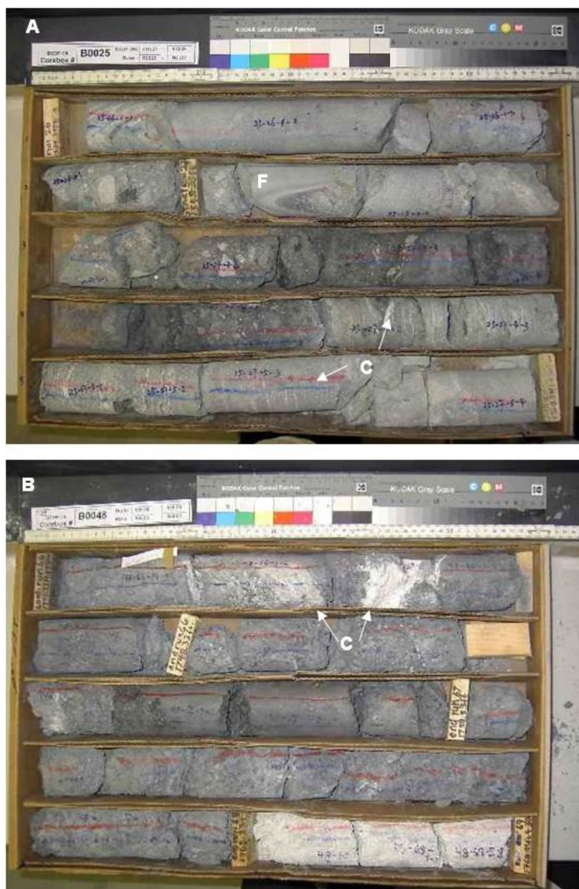
Fig. 3.6: Pre- and post-impact alteration. A) Core box image of secondary carbonate veins (C) and a fold structure (F) in suevites of upper impactites (Box no. 25, depth range = 410.21 - 413.04 m). B) Core box image of carbonate pods (C) in shales of the basement metasediments (Box no. 48, depth range = 530.39 – 539.29 m).
