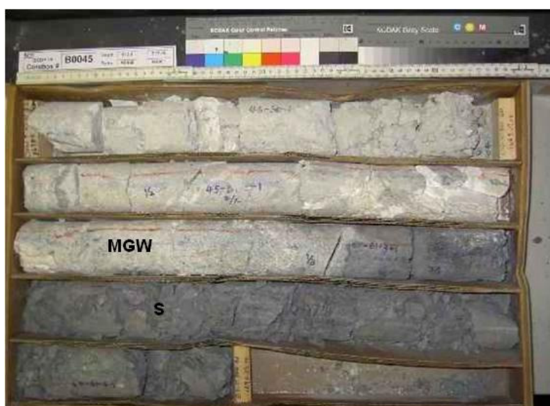
Fig. 3.4: Core box image of basement metasediments (Box no. 45, depth range = 512.80 – 517.65 m) indicating the difference between the metagreywacke (MGW)-rich sediments (light grey), and the shale (S)-rich sediments (dark grey). Horizontal length of core box is 60 cm.
