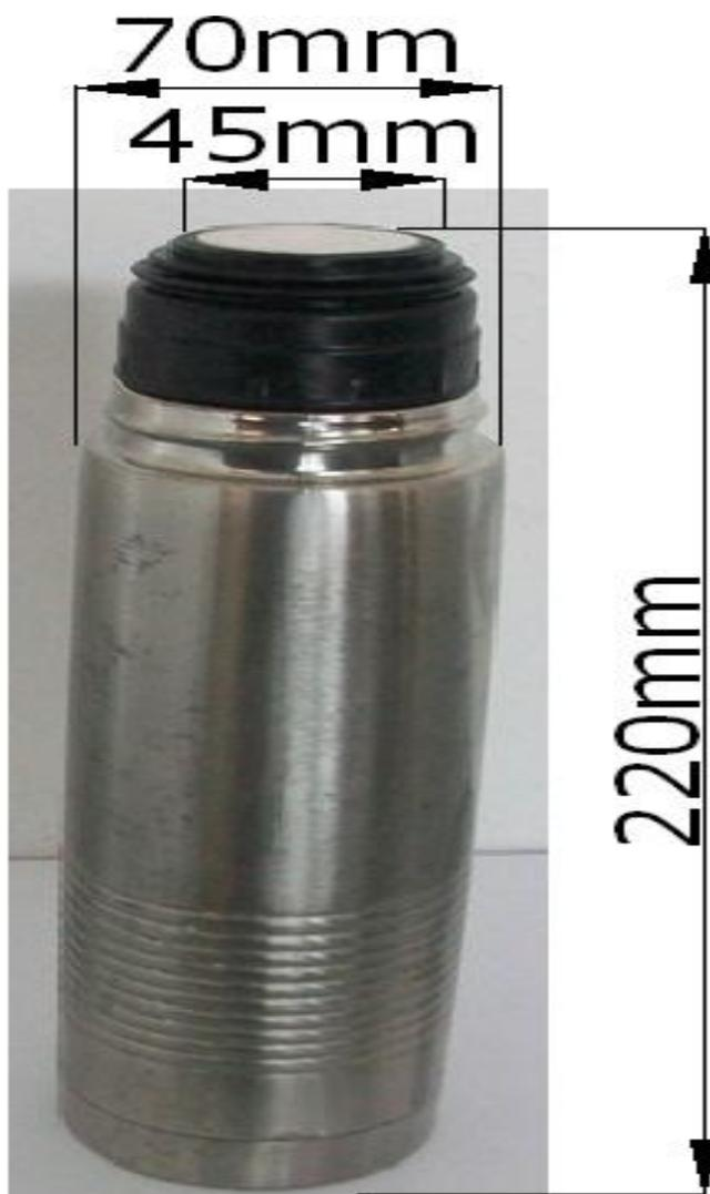
**Figure (3.5): The reaction vessel**
