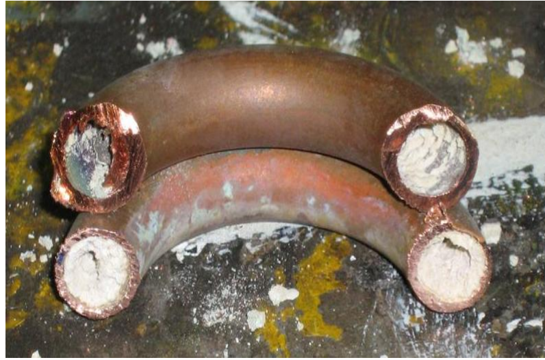
Figure 2-4 Heat exchanger tubes clogged up with \text{CaCO}_3 precipitated solids
