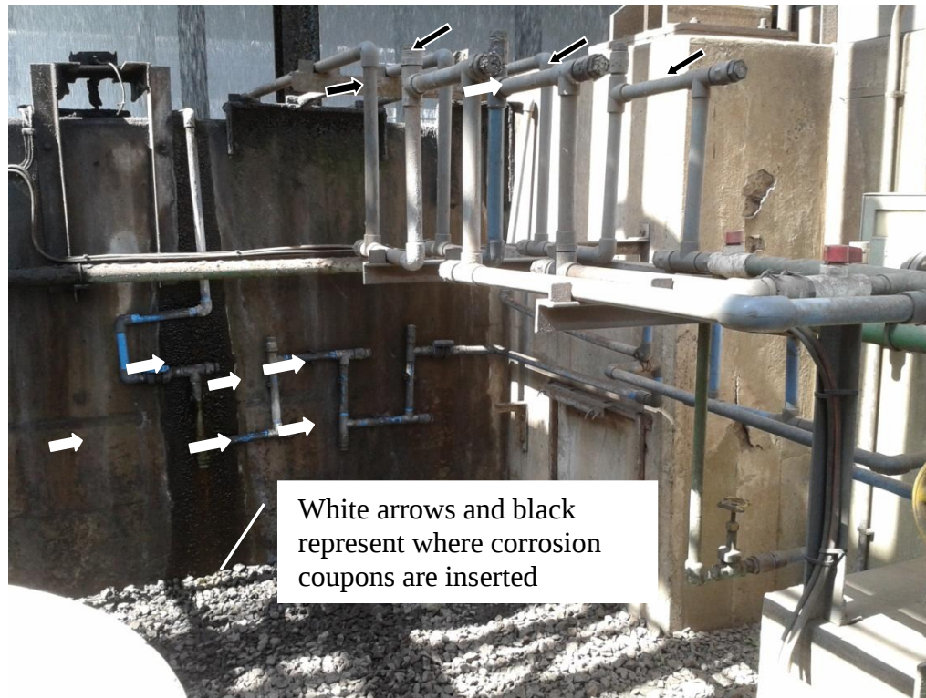
Figure 3-5 Corrosion coupon insertion points
