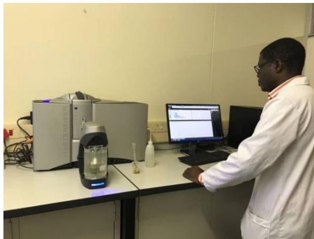
Figure 3.6: Determination of soil particle size distribution using laser diffraction, Mastersizer 3000.
