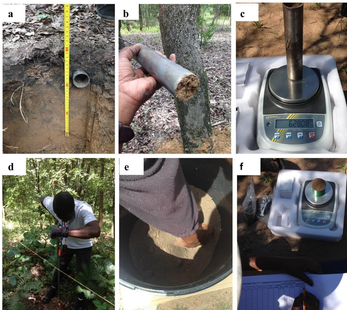
Figure 3.5: Forest soil sampling in Luanshya and Bushbuckridge. The figure shows (a, b) core sampling method and (c) determination of field or wet mass of undisturbed soil, and (d) auger sampling method, (e) compositing soil of the same depth and plot and (f) weighing of wet soil using a field electronic balance.
