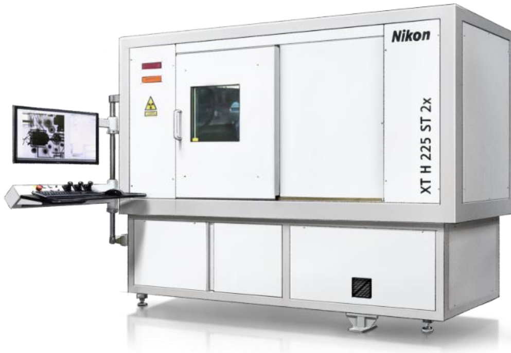
Figure 3.2: Nikon XTH/225 Micro-focus X-Ray tomography scanner ( https://industry.nikon.com/en-us/products/x-ray-ct/ ).
